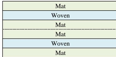
Fig. 2 The stacking sequence of composite samples
