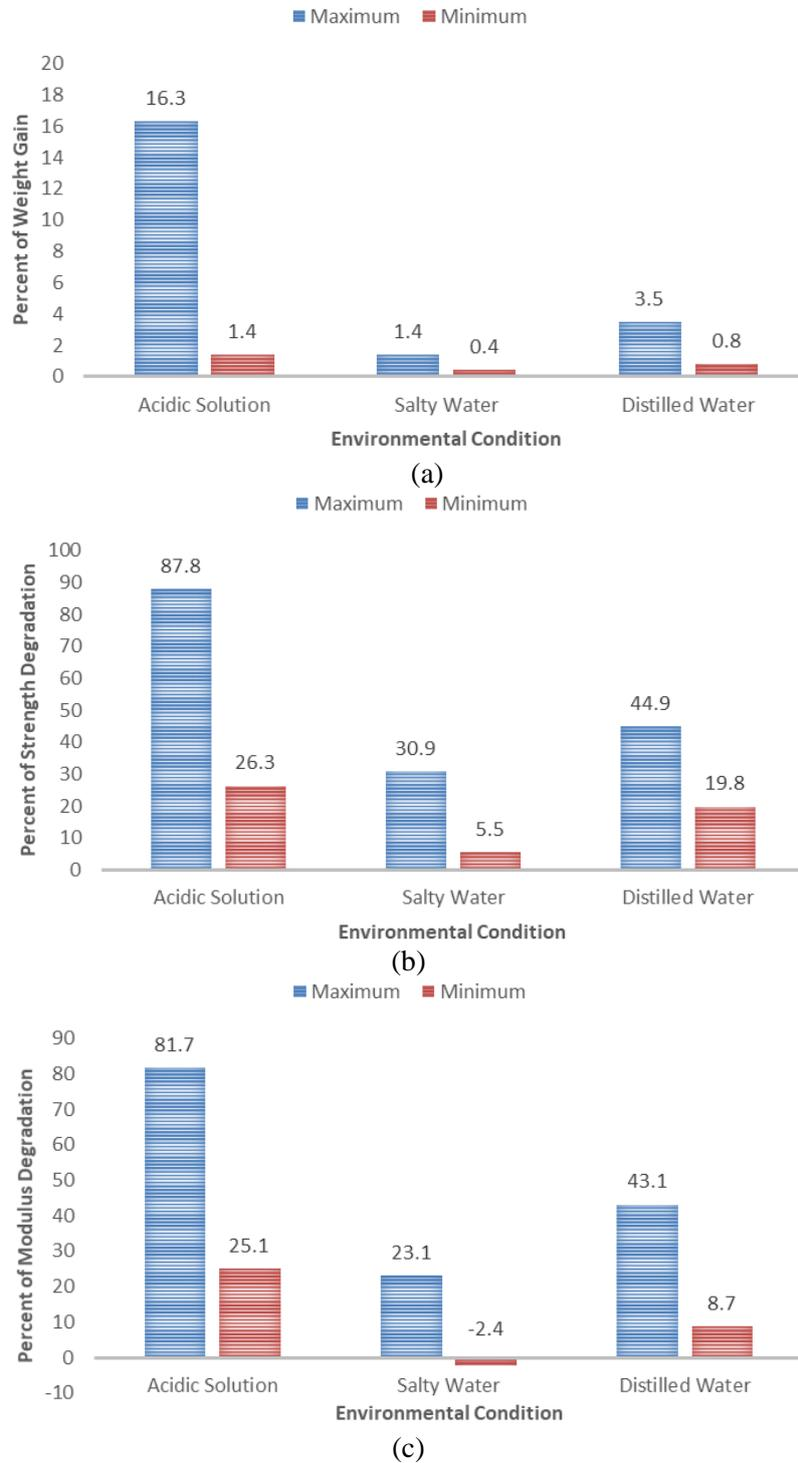
Fig. 8 The minimum and maximum values of aged samples immersed in three environmental conditions a) weight change, b) flexural strength, c) flexural modulus
