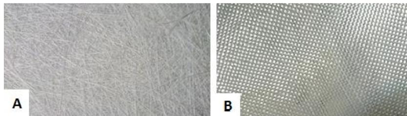
Fig. 1 The ECR glass fibers used for the fabrication of composite specimens A) chopped strand mat and B) woven fabric
