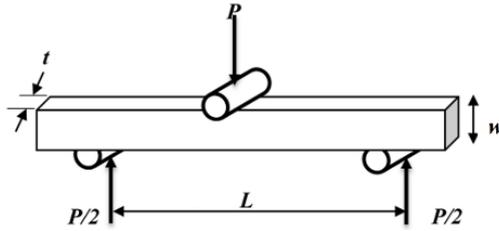
Fig. 4 A schematic of the three-point bending test
