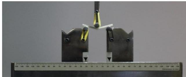
Fig. 3 The three-point bending test fixture
