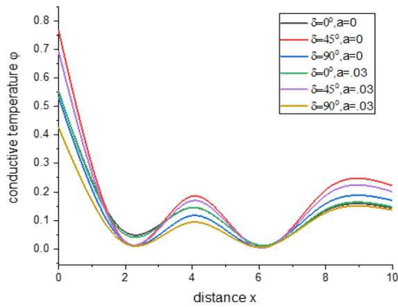
Fig. 5 variation of conductive temperature  $\phi$  with the distance  $x$  (uniformly distributed force)
