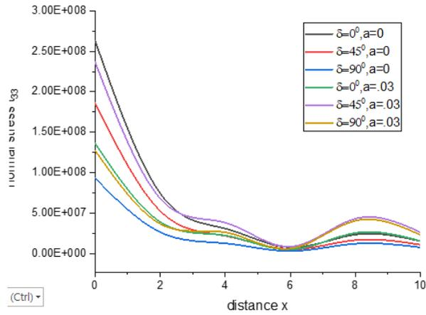
Fig. 6 variation of normal stress  $t_{33}$  with the distance  $x$  (uniformly distributed force)
