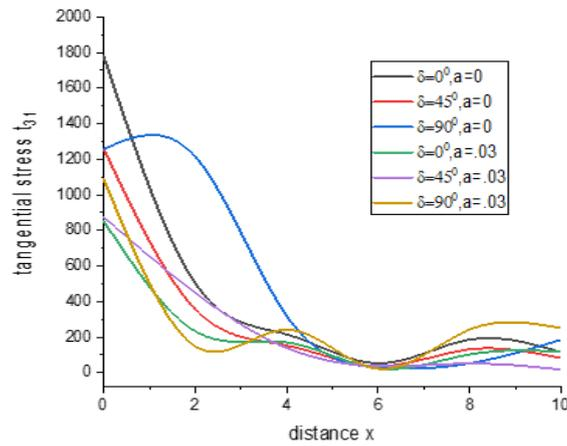
Fig. 7 variation of tangential stress  $t_{31}$  with the distance  $x$  (uniformly distributed force)
