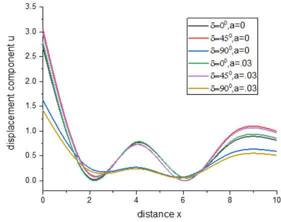
Fig. 3 variation of displacement component  $u$  with the distance  $x$  (uniformly distributed force)
