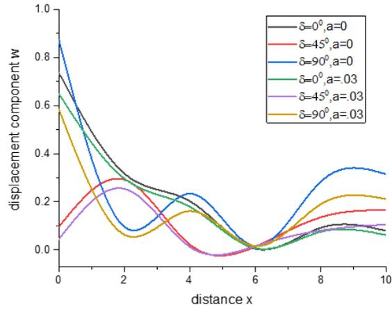
Fig. 4 variation of displacement component  $w$  with the distance  $x$  (uniformly distributed force)
