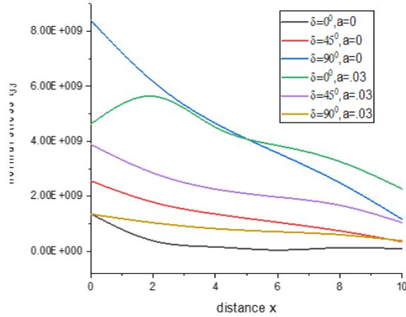
Fig. 12 variation of normal stress  $t_{33}$  with the distance  $x$  (linearly distributed force)
