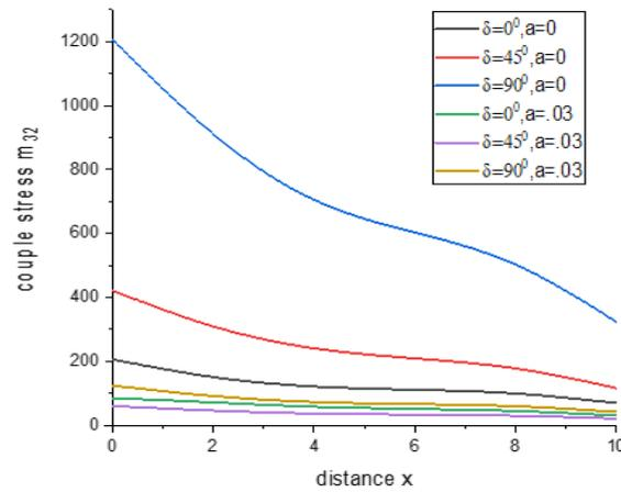
Fig. 14 variation of couple stress  $m_{32}$  with the distance  $x$  (linearly distributed force)
