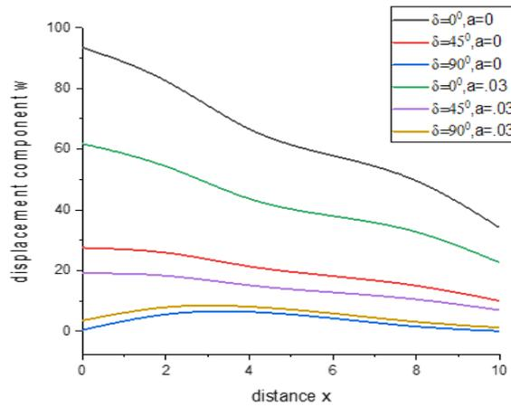
Fig. 10 variation of displacement component  $w$  with the distance  $x$  (linearly distributed force)
