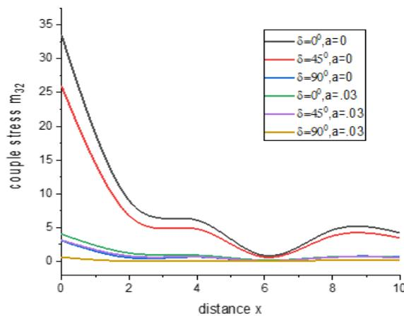
Fig. 8 variation of couple stress  $m_{32}$  with the distance  $x$  (uniformly distributed force)
