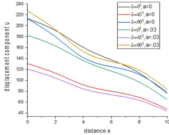
Fig. 9 Variation of displacement component  $u$  with the distance  $x$  (linearly distributed force)
