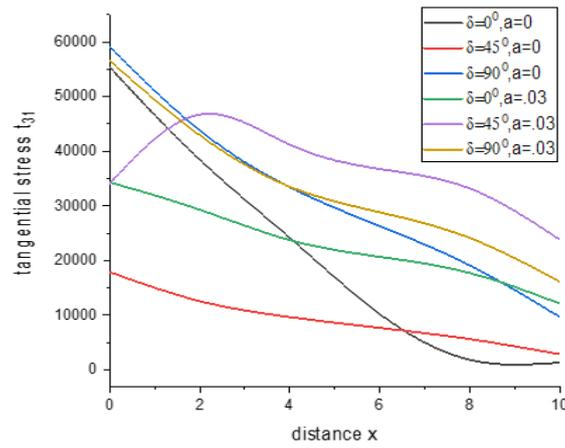
Fig. 13 variation of tangential stress  $t_{31}$  with the distance  $x$  (linearly distributed force)
