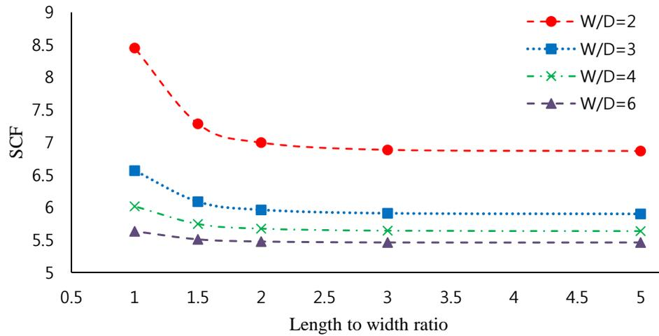
Fig. 3 SCF against length to width ratio for  $(0_2/90)_s$  Laminate
