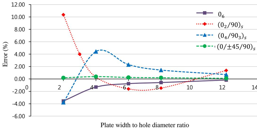
Fig. 10 Error of Eq. (26) versus plate width to hole diameter ratio ( $\lambda = 1$ )
