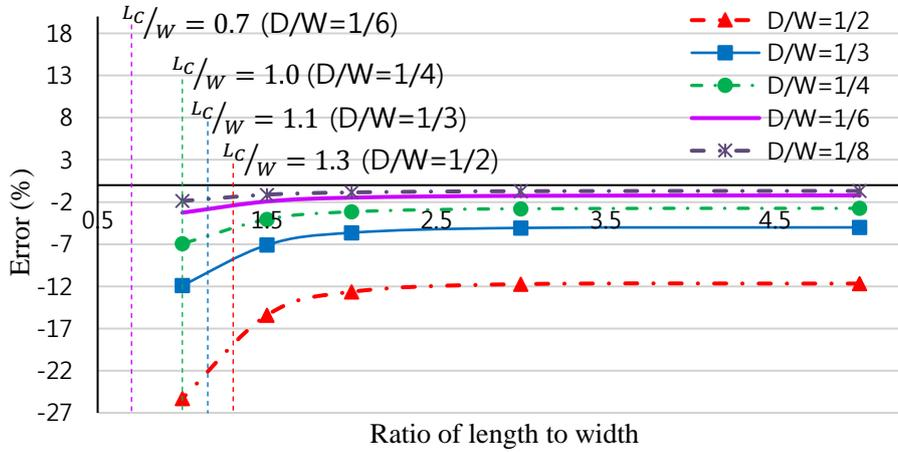
Fig. 7 Error of SCFs obtained from the exact solution (Eq. (1)) against length to width ratio for  $(0_4/\pm 45/90_2)_s$  laminate
