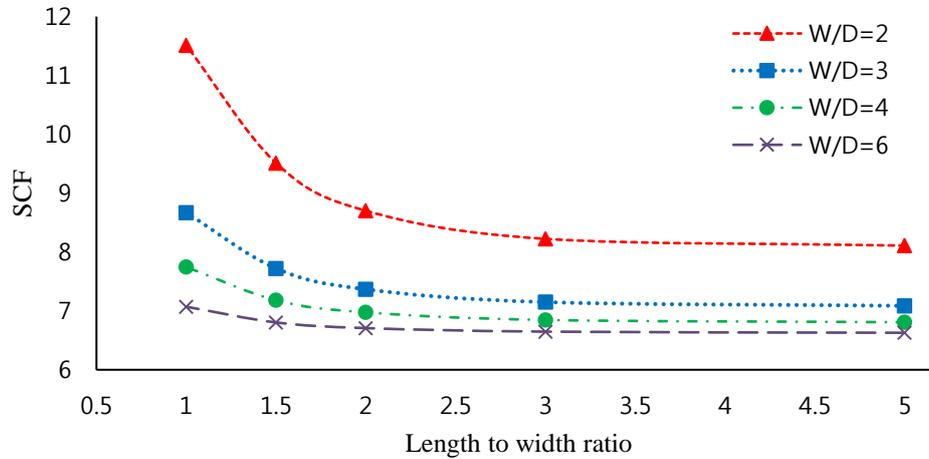
Fig. 2 SCF against length to width ratio for  $0_6$  Laminate
