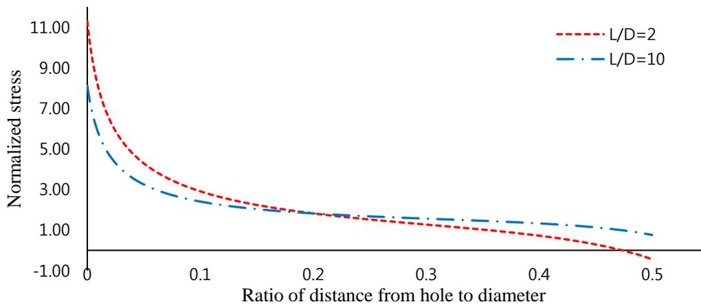
Fig. 4 Normalized stress distribution of a  $0_6$  laminate with  $width/diameter = 2$  along line  $\overline{AB}$
