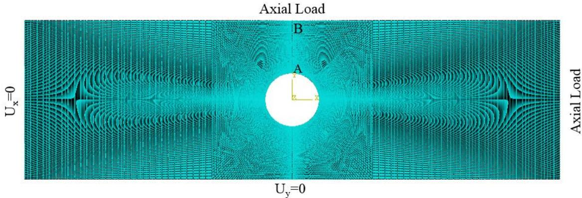
Fig. 9 An exemplary meshed model and general B.C. of biaxial loading
