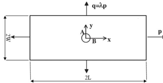
Fig. 8 A finite plate under biaxial loading
