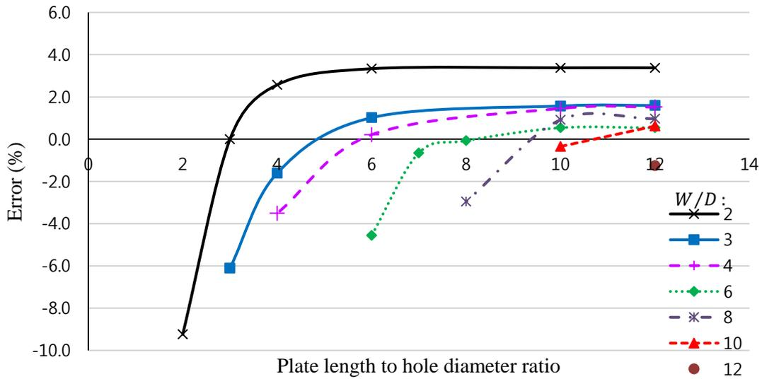
Fig. 14. Error of the basic exact solution (Eq. (22)) versus length to diameter ratio in  $(0_2/90)_s$  laminates with  $\lambda = 1$
