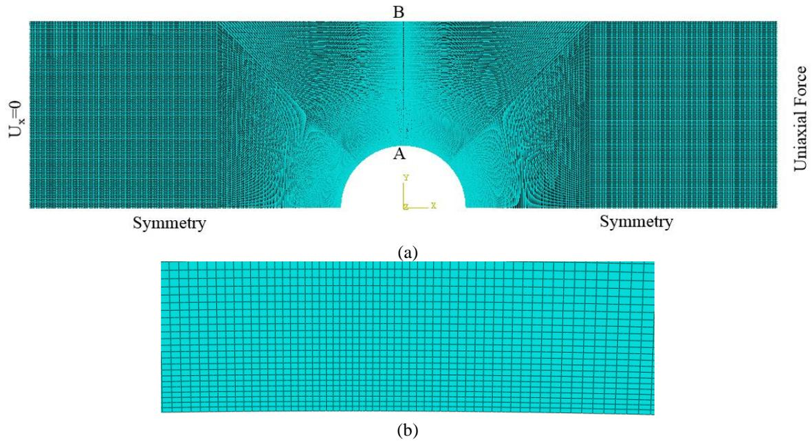
Fig. 1 A: an exemplary meshed geometry and the general B.C. of uniaxial loading, B: Magnification around point “A”
