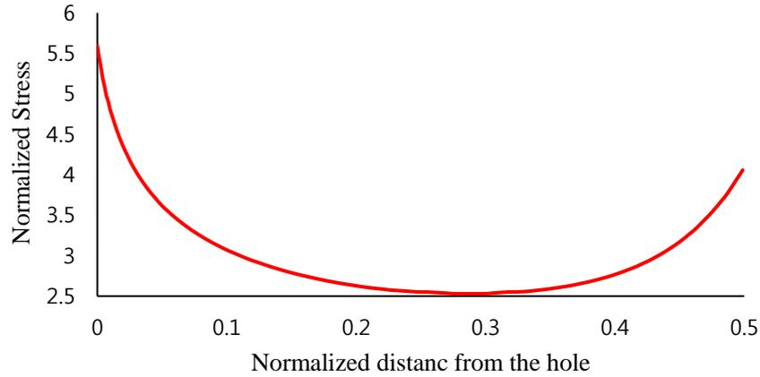
Fig. 11 Stress profile of the  $(0_2/90)_s$  laminate with  $width/diameter = 2$  and  $\lambda = 1$  along the line  $\overline{AB}$
