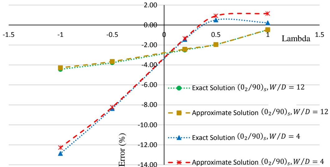
Fig. 12 Error versus lambda for  $(0_2/90)_s$  laminates
