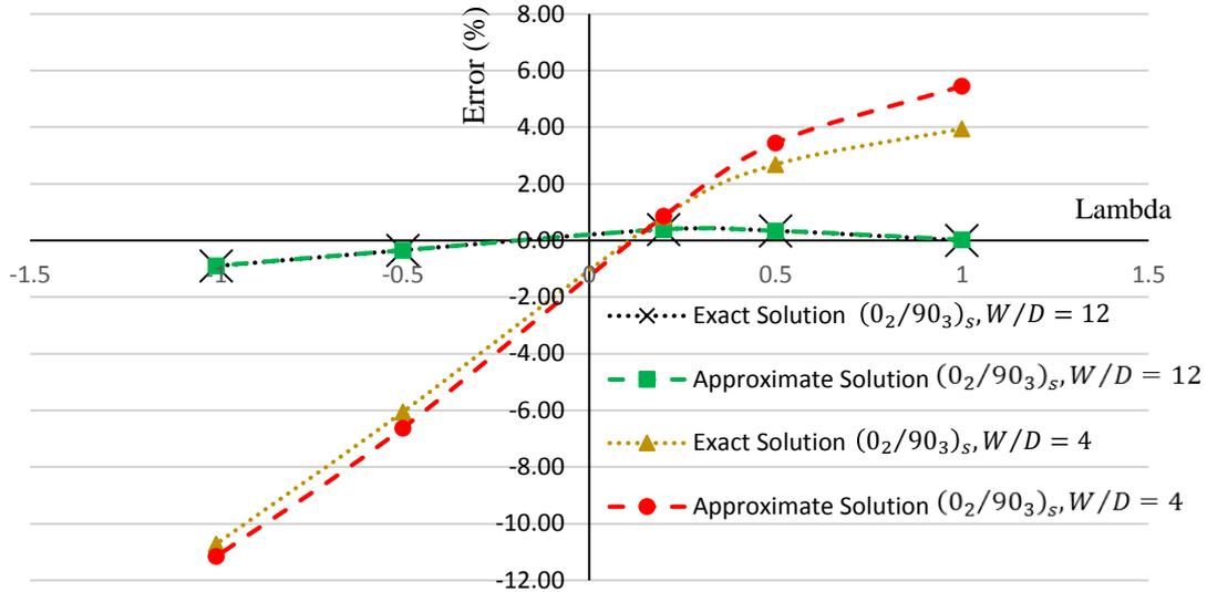
Fig. 13. Error versus lambda for  $(0_2/90_3)_s$  laminates
