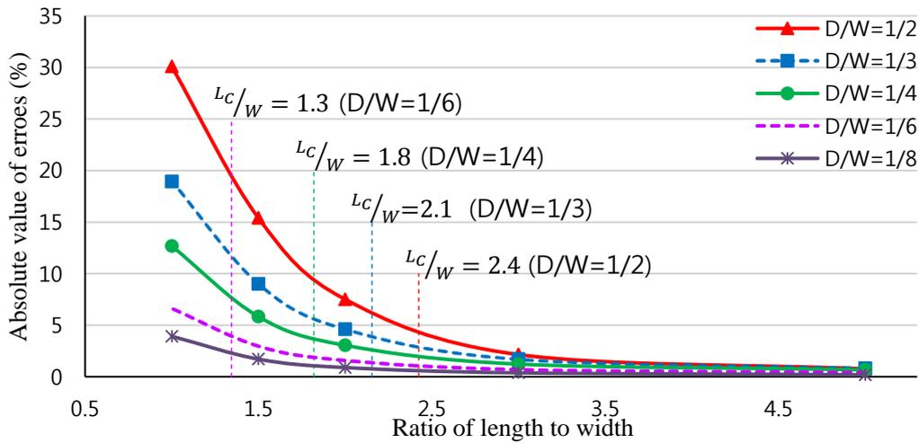
Fig. 5 Error of SCFs obtained from the exact solution (Eq. (1)) against length to width ratio for  $0_6$  laminate
