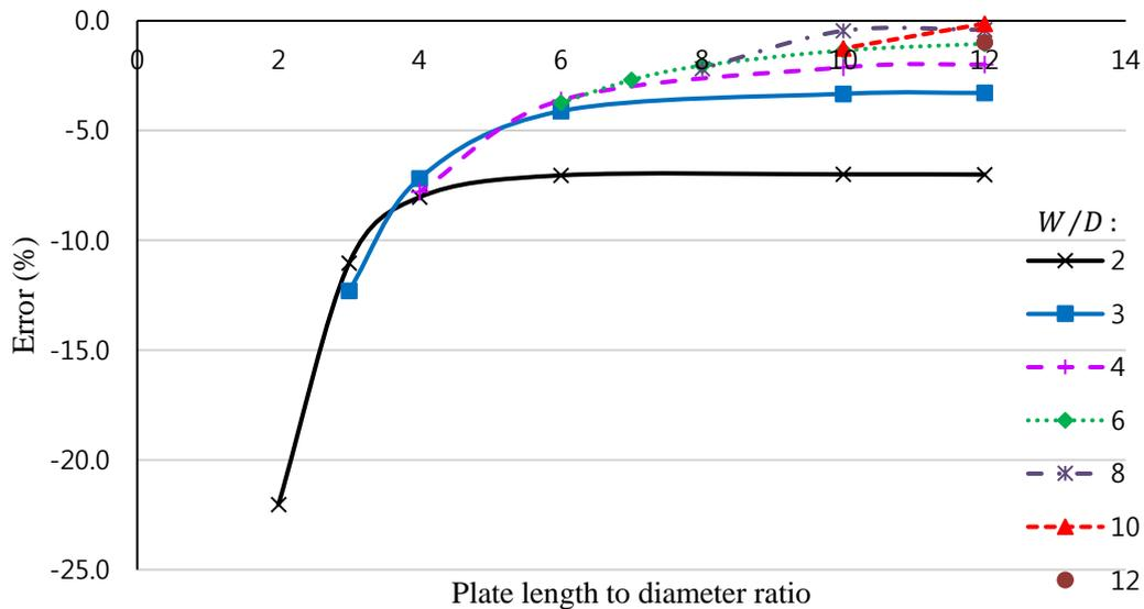
Fig. 15. Error of the improved exact solution (Eq. (26)) versus length to diameter ratio in  $(0_2/90)_s$  laminates with  $\lambda = -0.5$
