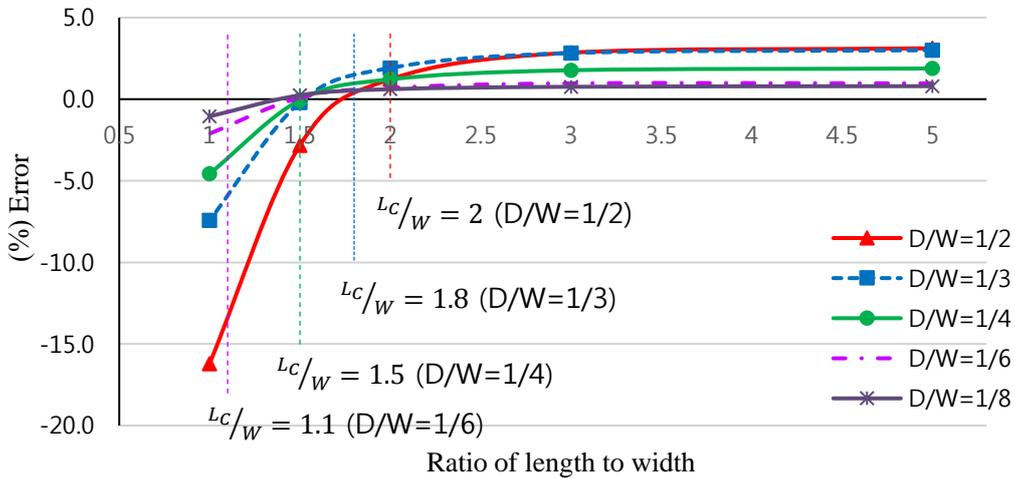
Fig. 6 Error of SCFs obtained from the improved approximate solution (Eq. (4)) against length to width ratio for  $(0_2/90)_s$  laminate
