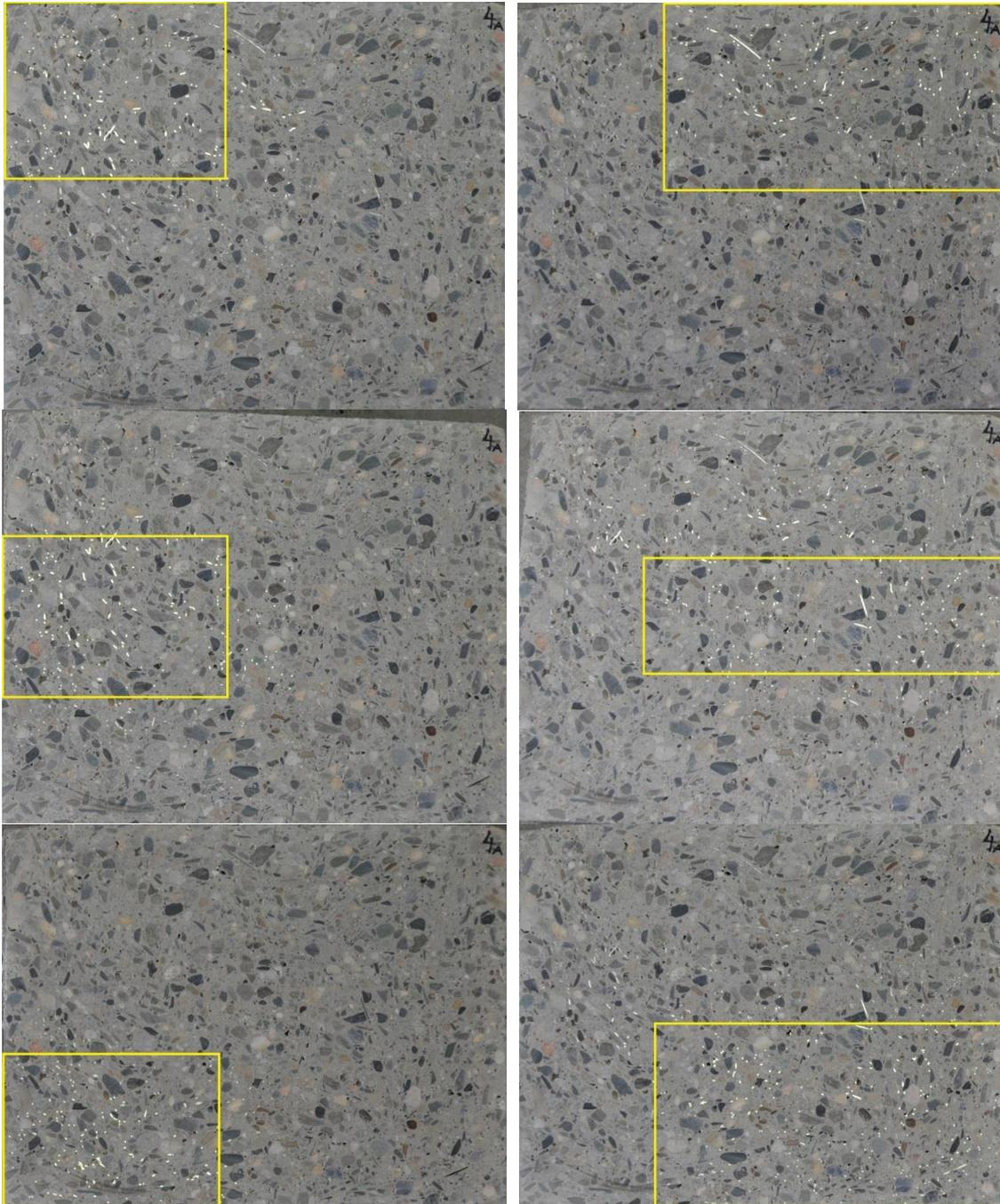
Fig. 12 Source images of cross-section of specimen 4A. Selected areas are highlighted by yellow lines
