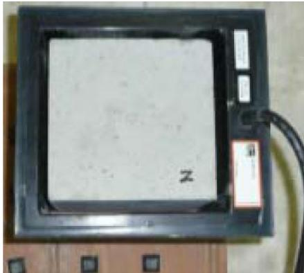
(a) SFRC sample in the coil (reprinted from Vitek *et al.* 2013)
