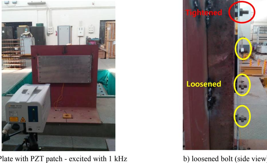
Fig. 10 Experiment set up for the bolt loosening
