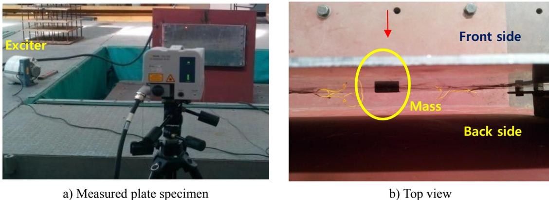
Fig. 7 Experimental setup for damage detection using SLVD
