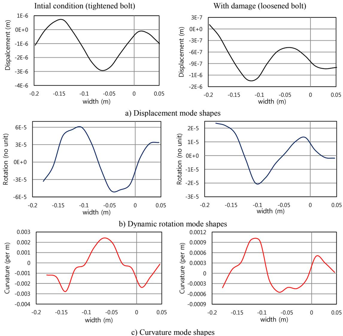
Fig. 12 Experimental results along plate width for bolt loosening problem
