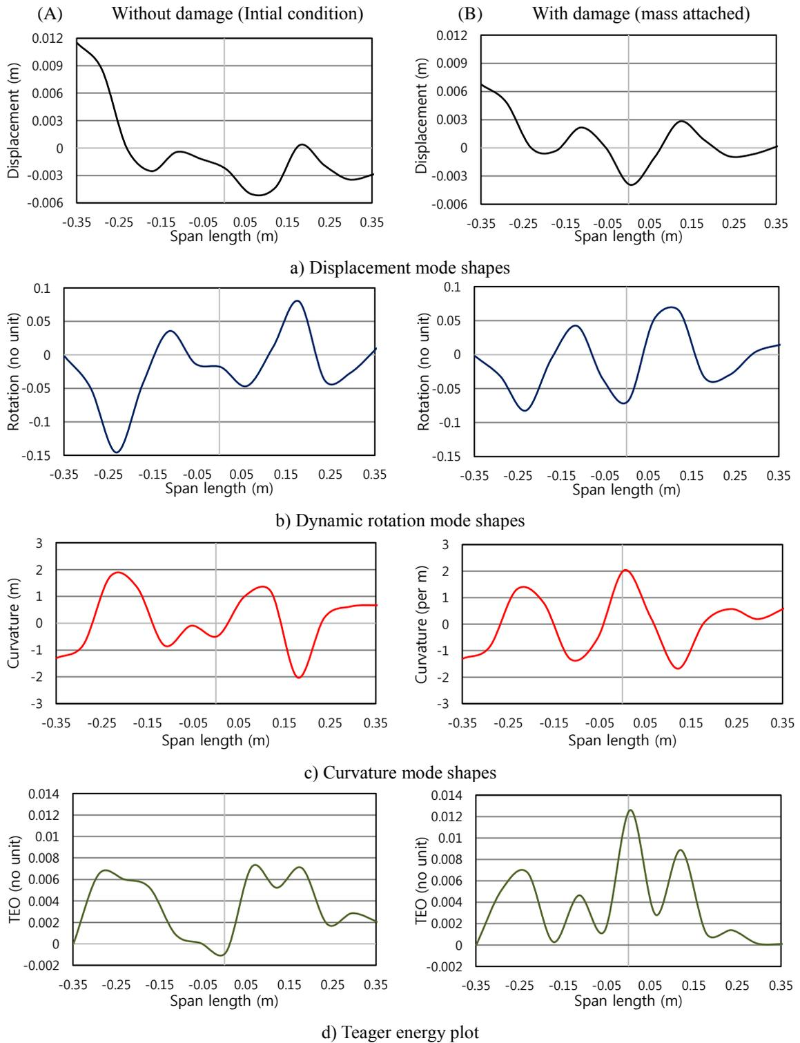
Fig. 9 Obtained from SLDV for sixth natural frequency of the plate (382.5 Hz - antisymmetric mode)
