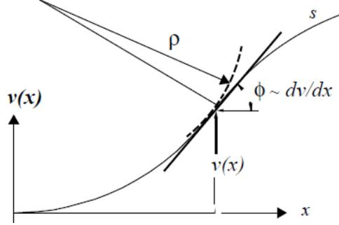
Fig. 1 Curvature of the deformed neutral axis (Bucciarelli 2009)
