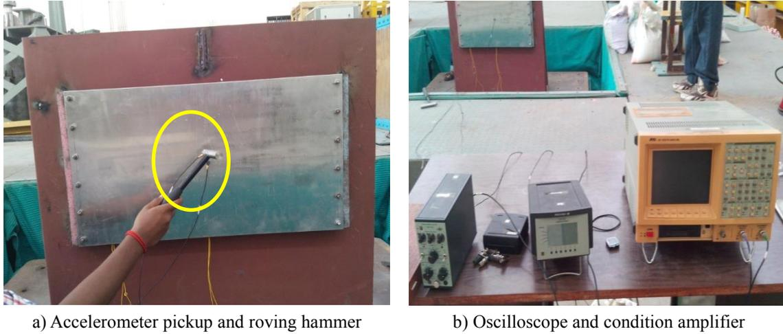
a) Accelerometer pickup and roving hammer
