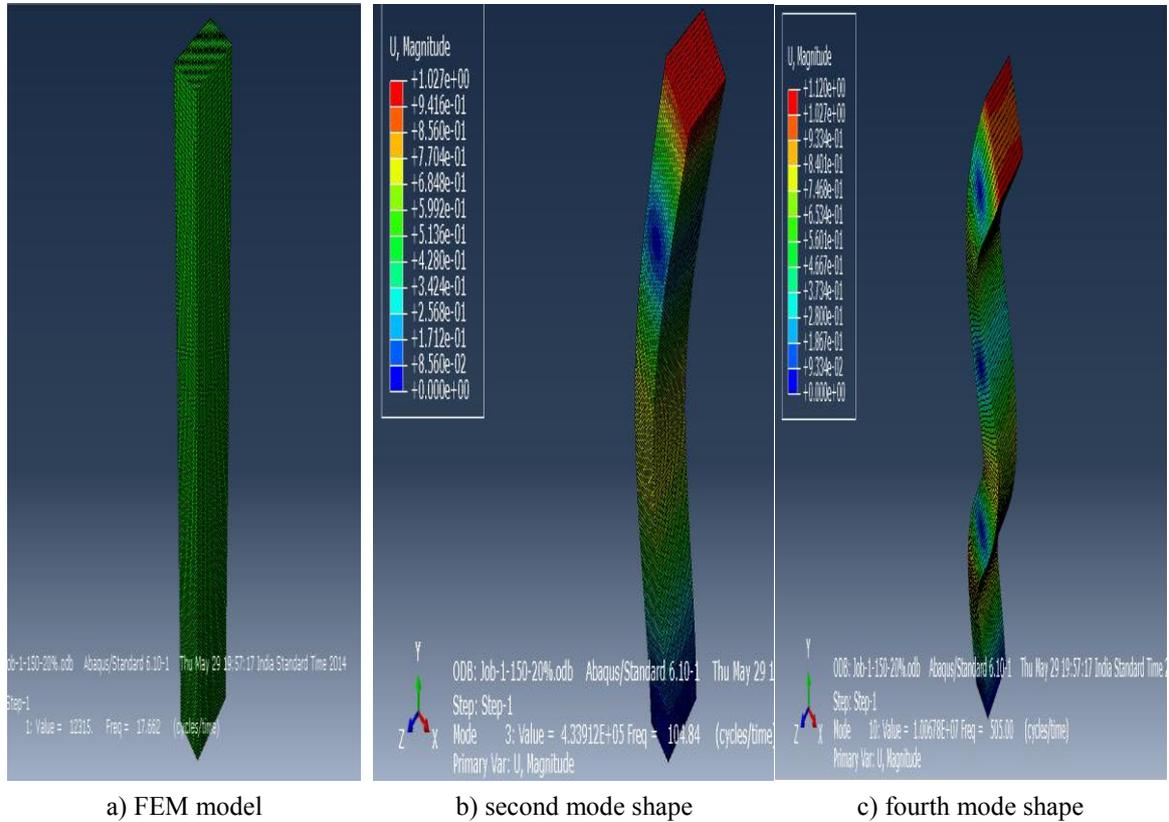
Fig. 2 SRC cantilever beam model
