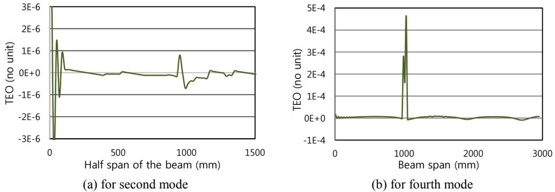
Fig. 4 Teager energy plot for cantilever beam with induced damage
