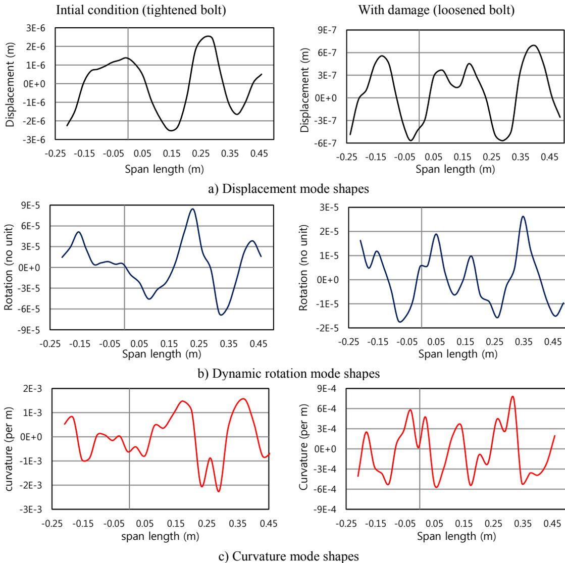
Fig. 11 Experimental results along plate span length for bolt loosening problem
