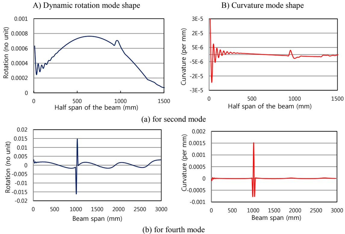
Fig. 3 Analytical results for SRC cantilever beam with induced damage
