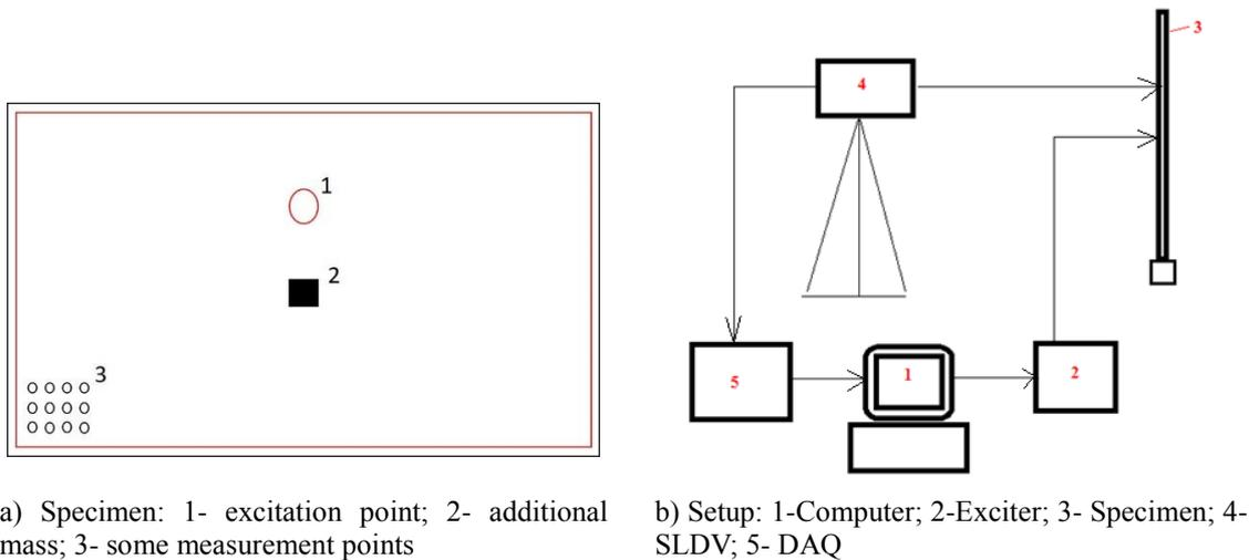
Fig. 6 Schematic view of measurement setup
