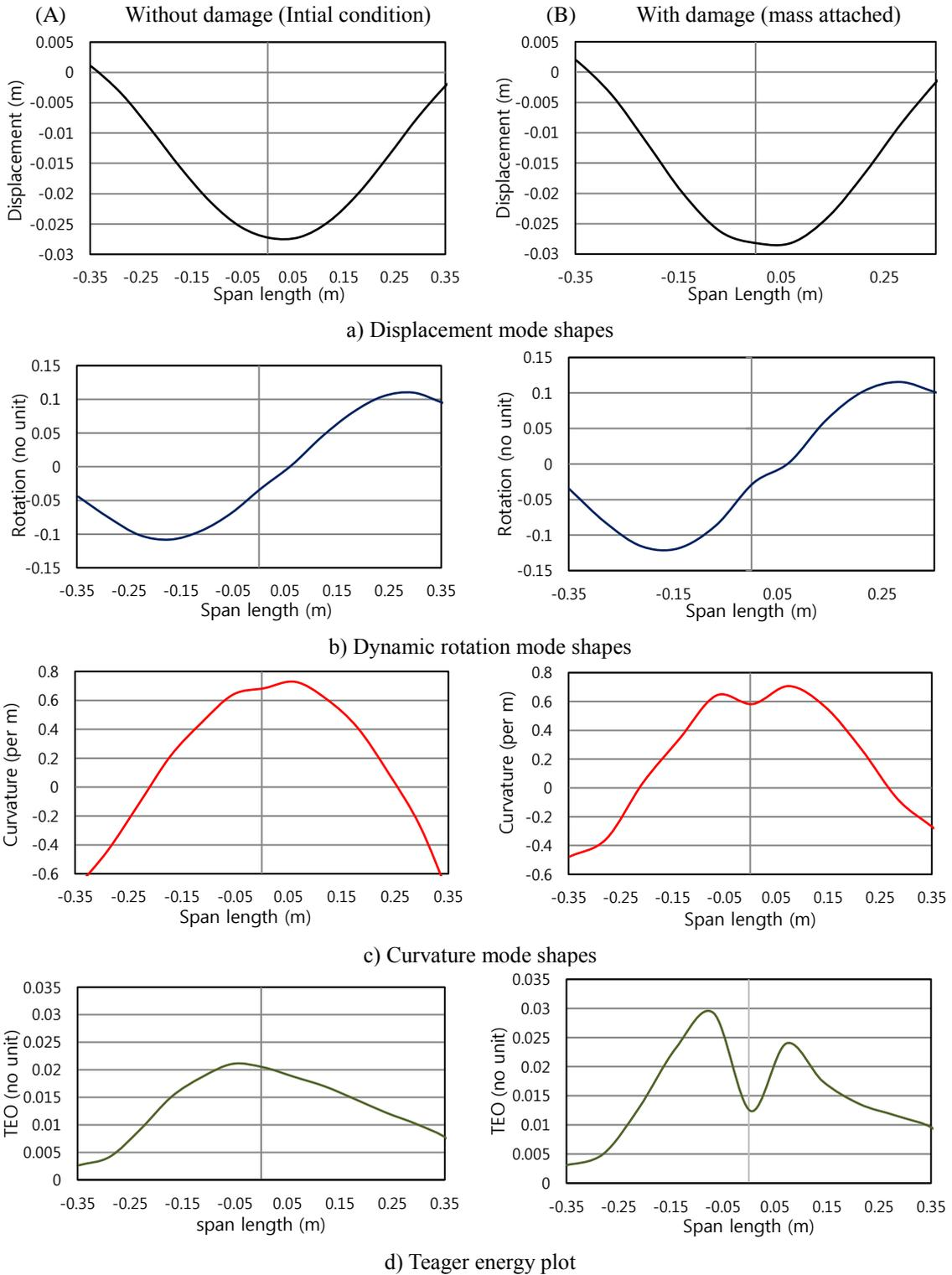
Fig. 8 Obtained from SLDV for first natural frequency of the plate (26.25 Hz - symmetric mode)
