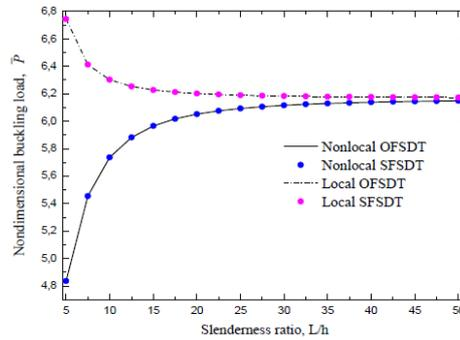
Fig. 3 Effect of the length to thickness ratio on dimensionless buckling load for  $k = 1$ ,  $e_0a = 1$  nm
