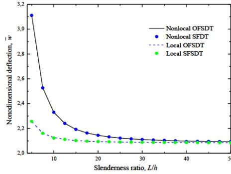
Fig. 2 Effect of the length to thickness ratio on dimensionless deflection for uniform load for  $k = 1$ ,  $e_0a = 1$  nm
