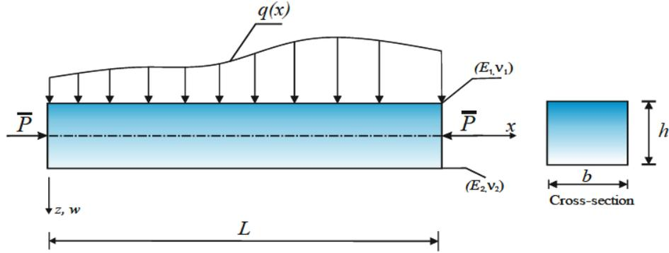
Fig. 1 Geometry and coordinates of functionally graded nano beam
