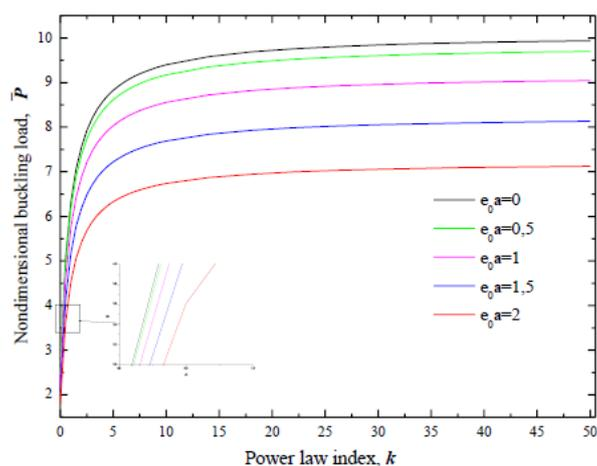
Fig. 7 Variation of the nondimensional buckling load of S-S FGM nanobeam with material gradation and for different scale parameter rises ( $L/h = 10$ )
