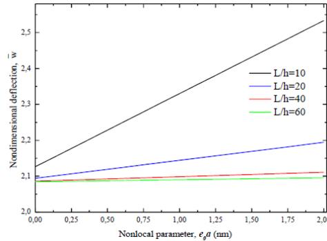
Fig. 4 Effect of nonlocal parameter on dimensionless deflection under uniform load for  $k = 1$
