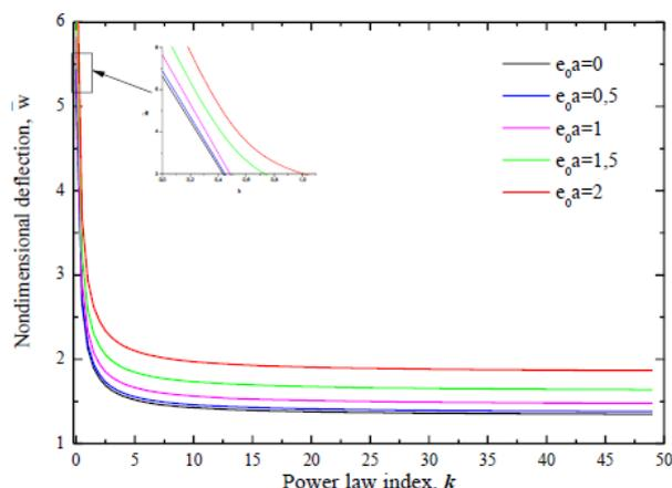
Fig. 6 Variation of the nondimensional deflection of S-S FGM nanobeam with material gradation and for different scale parameter rises ( $L/h = 10$ )
