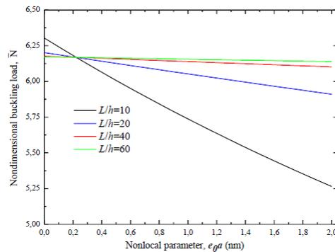
Fig. 5 Effect of nonlocal parameter on nondimensional buckling load for  $k = 1$
