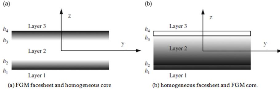
Fig. 2 The material variation along the thickness of the FGM sandwich plate
