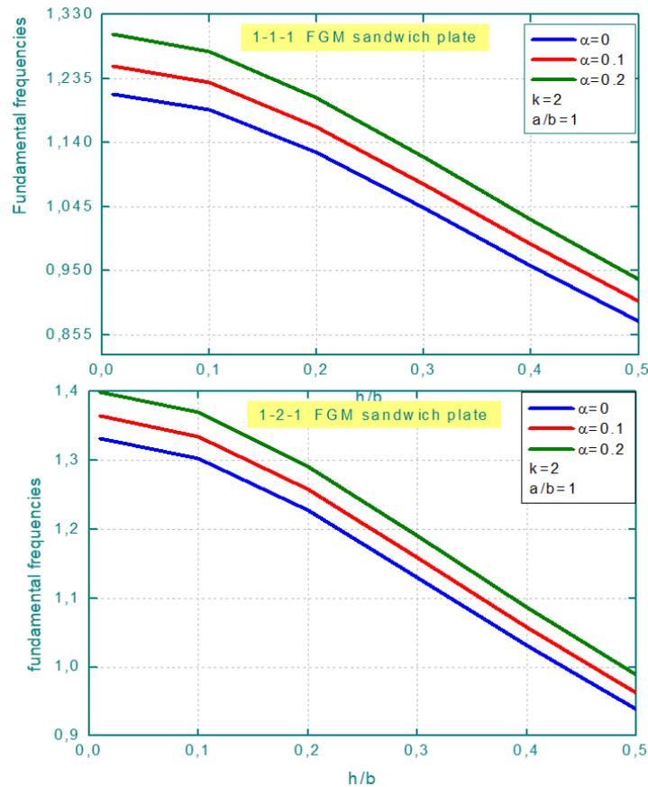
Fig. 3 Porosity influence on the dimensionless frequency versus the thickness ratio  $h/b$  for FGM sandwich plate with homogeneous hardcore
