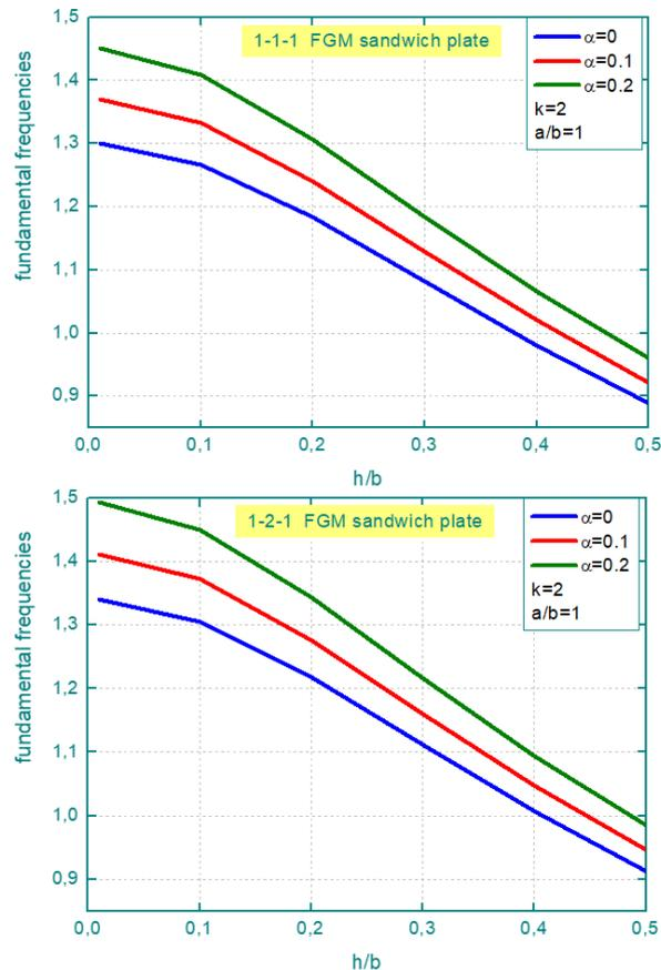
Fig. 5 Porosity influence on the dimensionless frequency versus the thickness ratio  $h/b$  for FGM sandwich plate with FGM core
