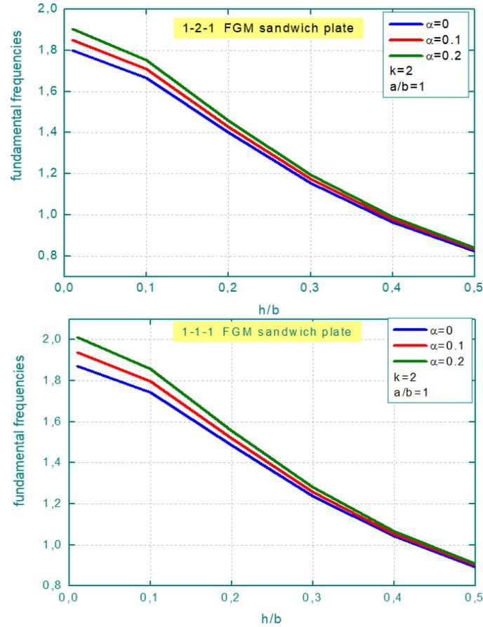
Fig. 4 Porosity influence on the dimensionless frequency versus the thickness ratio  $h/b$  for FGM sandwich plate with homogeneous soft-core
