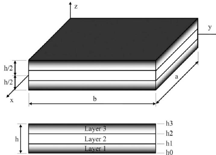
Fig. 1 The geometry of FGM sandwich plate
