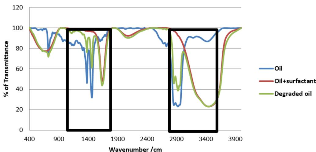
Fig. 15 Difference between the peaks of crude oil and degraded oil
