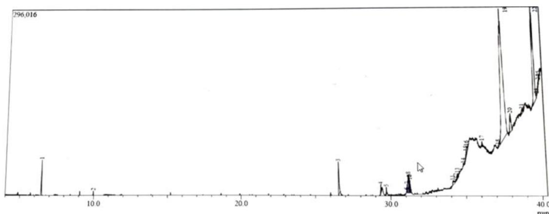
Fig. 16 Crude oil degradation in the presence of isolate *Bacillus subtilis*, 1% of crude oil as the solo carbon source
