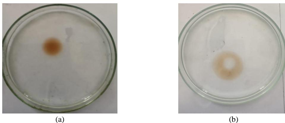
Fig. 6 (a) Crude Oil and (b) Crude Oil with surfactant
