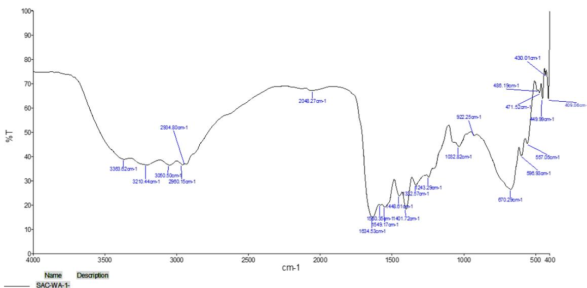
Fig. 14 FTIR spectra analysis of biosurfactant obtained from *B. subtilis*
