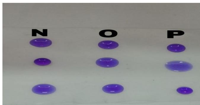
Fig. 12 Para film-M test (N-Distilled water, P-SDS, O-Sample)
