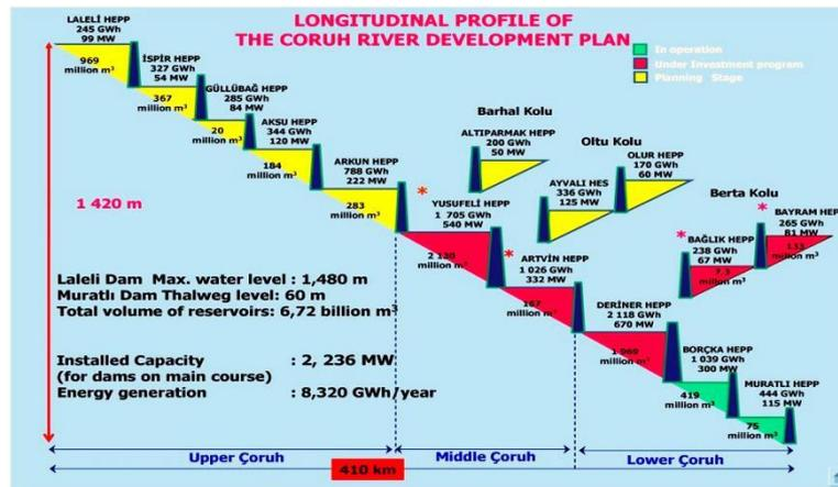
Fig. 1 Longitudinal profile of the Coruh River development plan
