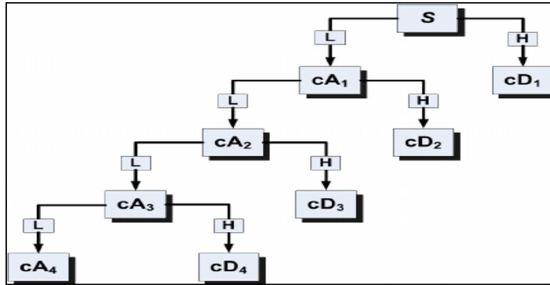
Fig 1 Wavelet Decomposition Tree upto 4<sup>th</sup> level
