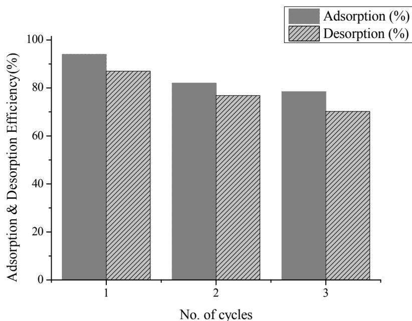
Fig. 6 Efficiency of the adsorption / desorption cycle
