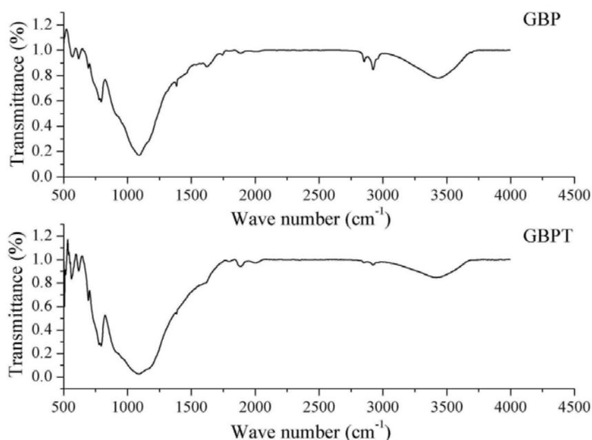
(a) Spectrum of GBP before adsorption (GBP) and after adsorption (GBPT)
