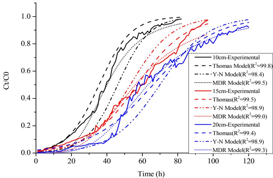
Fig. 2 Breakthrough curves from experiments (—) and models (---) at different bed heights ( $Q = 5 \text{ mL/min}$ ,  $C_0 = 15 \text{ mg/L}$ )
