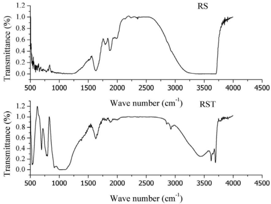
(b) Spectrum of RS before adsorption (RS) and after adsorption (RST)
