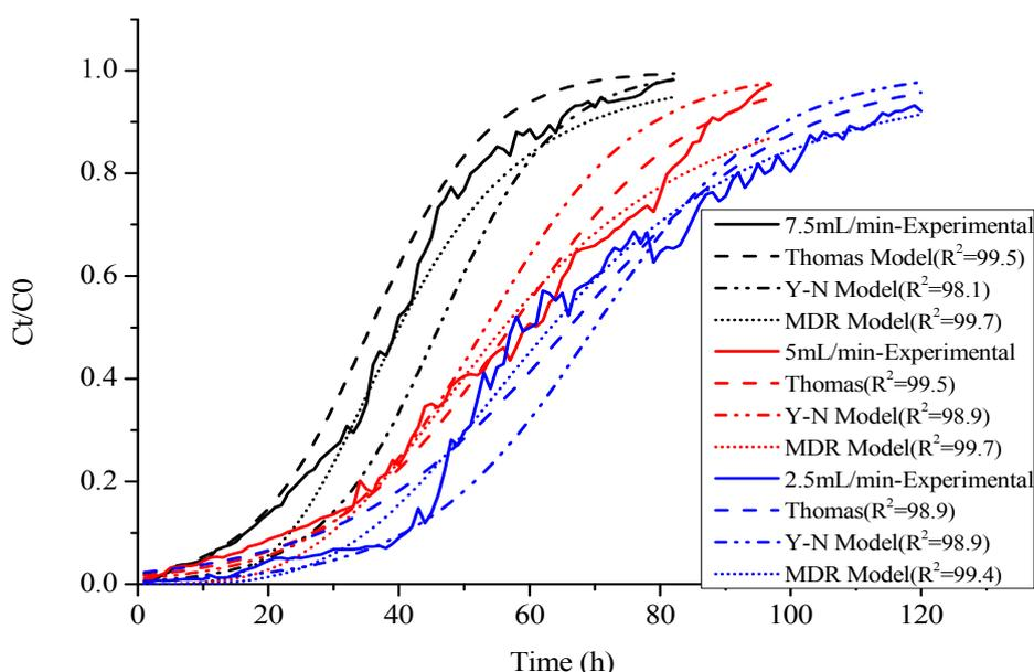
Fig. 3 Breakthrough curves from experiments (—) and models (---) at different flow rates (Bed height = 15 cm,  $C_0 = 15$  mg/L)
