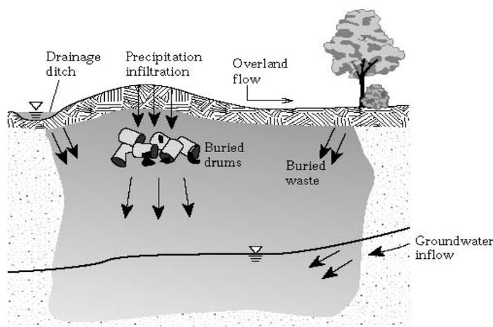
Fig. 1 Sources of fluid for the generation of landfill leachate
