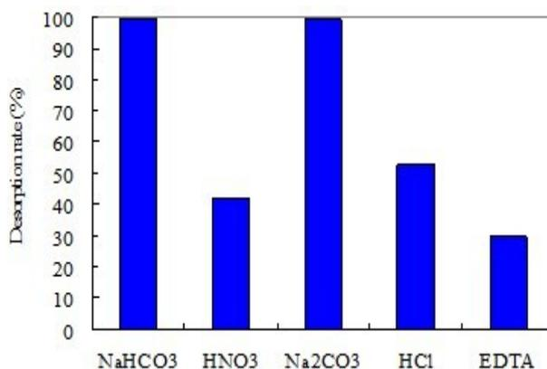
Fig. 9 Effect of different desorbents on desorption
