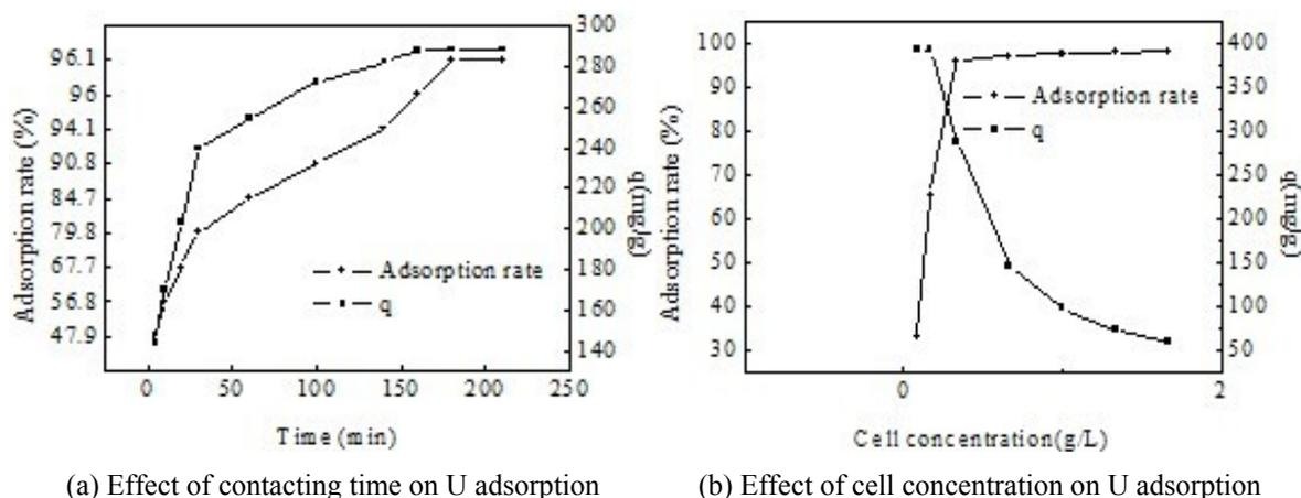
Fig. 7 Effect of contacting time and cell concentration on adsorption of U
