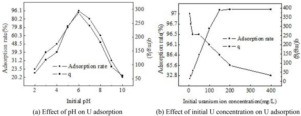
Fig. 6 Effect of initial pH and U concentration on adsorption U adsorption
