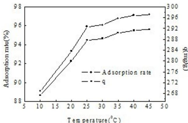
Fig. 8 Effect of temperature on U adsorption
