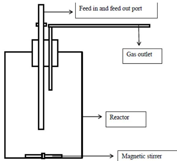
Fig. 2 CSTR schematic layout
