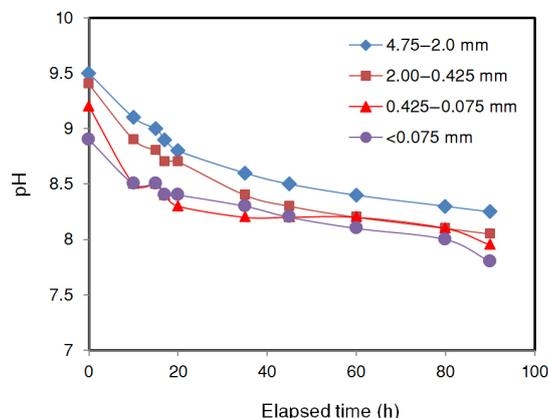
Fig. 3 Correlation in the pH of construction waste soil by particle size
