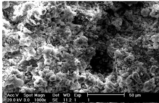
Fig. 2 Scanning electron microscope image of construction waste soil
