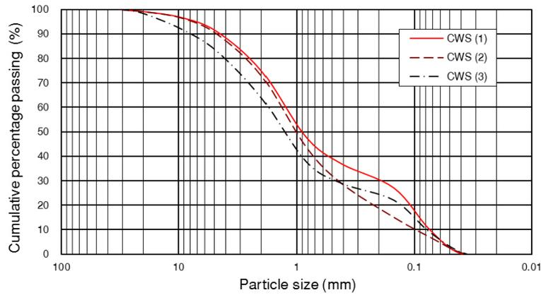
Fig. 1 Typical particle size distribution of construction waste soil
