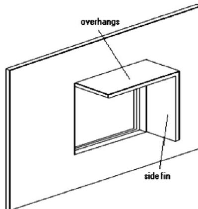
Fig. 2 Shading device configuration
