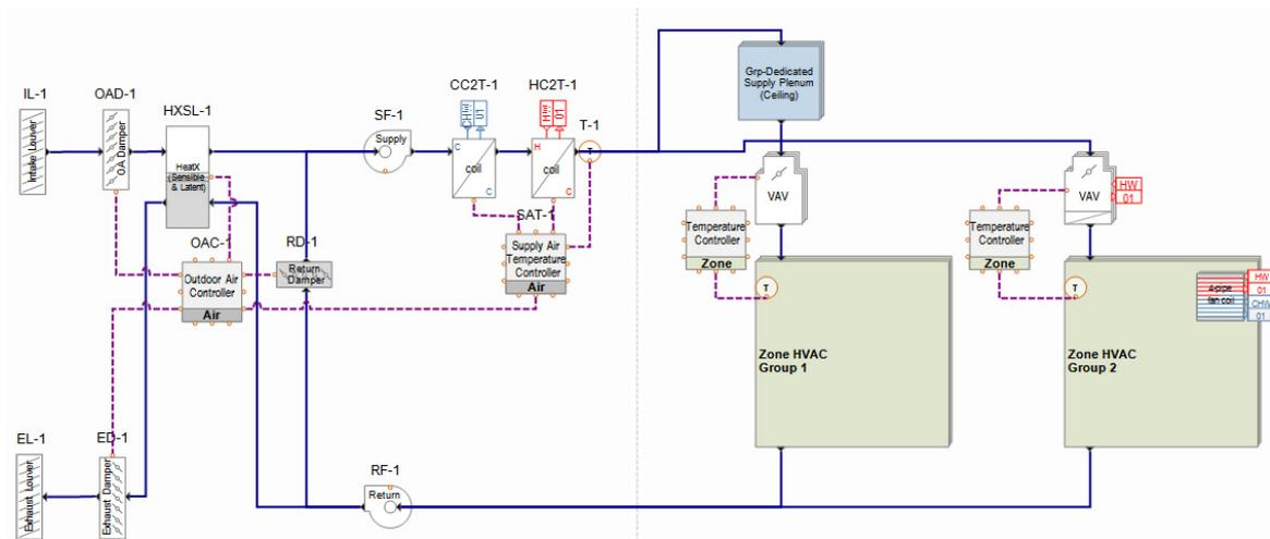
Fig. 5 Air loop block diagram
