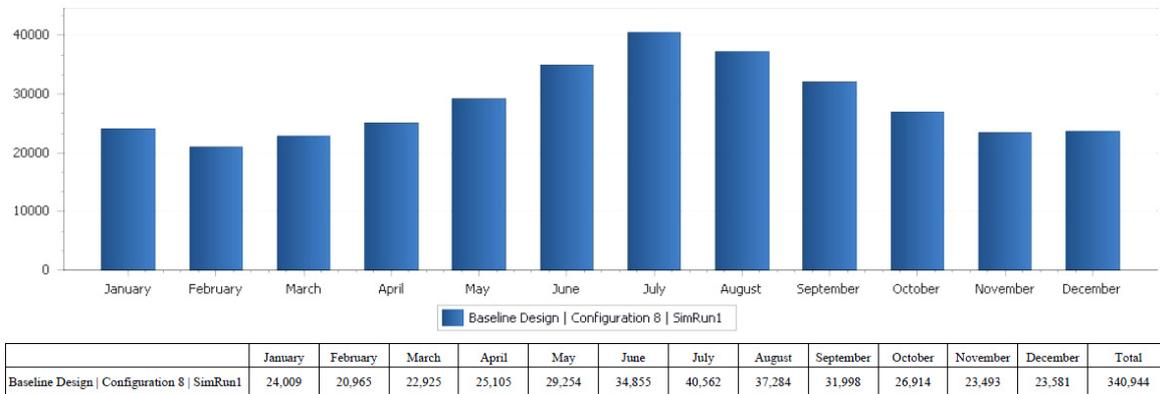
Fig. 9 Total monthly electrical consumption (kWh), After retrofit
