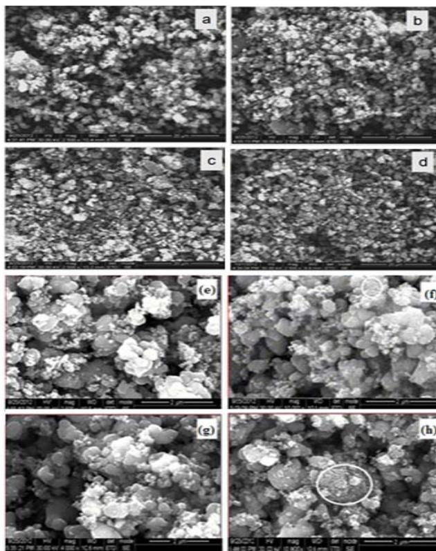
Fig. 2 SEM micrographs of (a)  $\text{Fe}_{0.2}\text{TiO}_2\text{NP}$  (b)  $\text{Fe}_{0.5}\text{TiO}_2\text{NP}$  (c)  $\text{Fe}_{1.0}\text{TiO}_2\text{NP}$  (d)  $\text{Fe}_{2.0}\text{TiO}_2\text{NP}$  (e)  $\text{C}_{2.0}\text{Fe}_{1.0}\text{TiO}_2\text{NP}$  (f)  $\text{C}_{2.0}\text{Fe}_{2.0}\text{TiO}_2\text{NP}$  (g)  $\text{C}_{4.0}\text{Fe}_{1.0}\text{TiO}_2\text{NP}$  (h)  $\text{C}_{4.0}\text{Fe}_{2.0}\text{TiO}_2\text{NP}$
