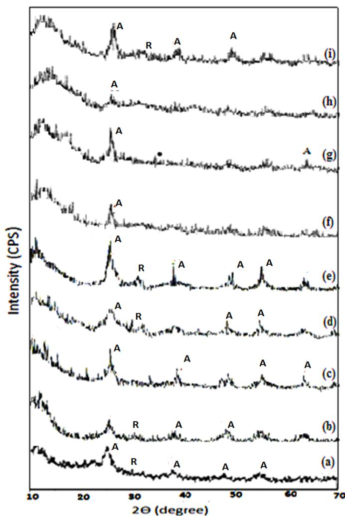
Fig. 1 X-ray diffraction patterns of (a) Pure  $\text{TiO}_2$  NP (b)  $\text{Fe}_{0.2}\text{TiO}_2\text{NP}$  (c)  $\text{Fe}_{0.5}\text{TiO}_2\text{NP}$  (d)  $\text{Fe}_{1.0}\text{TiO}_2\text{NP}$  (e)  $\text{Fe}_{2.0}\text{TiO}_2\text{NP}$  (f)  $\text{C}_{2.0}\text{Fe}_{1.0}\text{TiO}_2\text{NP}$  (g)  $\text{C}_{2.0}\text{Fe}_{2.0}\text{TiO}_2\text{NP}$  (h)  $\text{C}_{4.0}\text{Fe}_{1.0}\text{TiO}_2\text{NP}$  (i)  $\text{C}_{4.0}\text{Fe}_{2.0}\text{TiO}_2\text{NP}$
