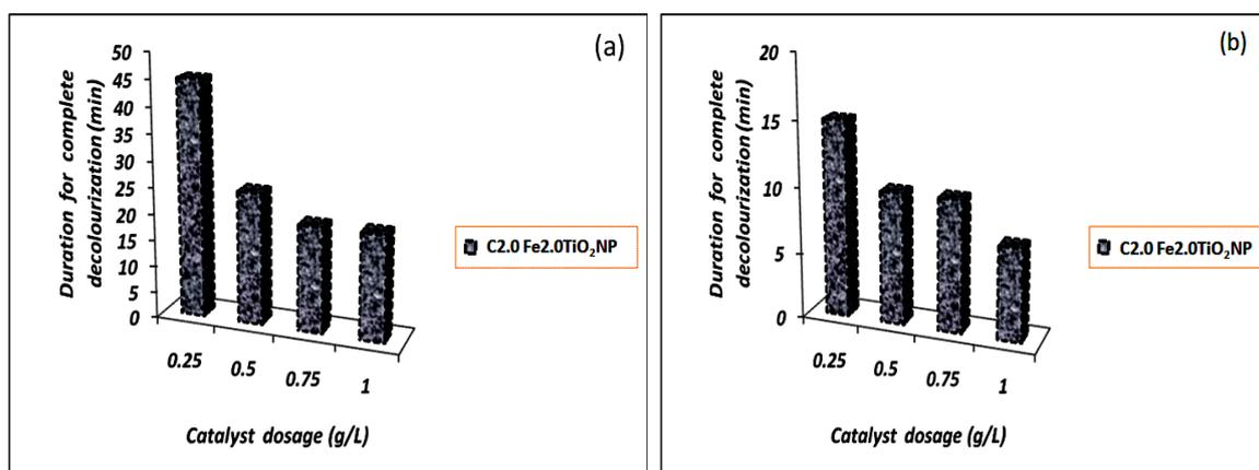
Fig. 8 Effect of catalyst dosage in the decolorization of (a) BB and (b) AO (Experimental conditions : Initial concentration of dye=10 ppm;  $\text{H}_2\text{O}_2$  concentration=29.7 mmol/L; Initial solar intensity ~55,000 LUX)
