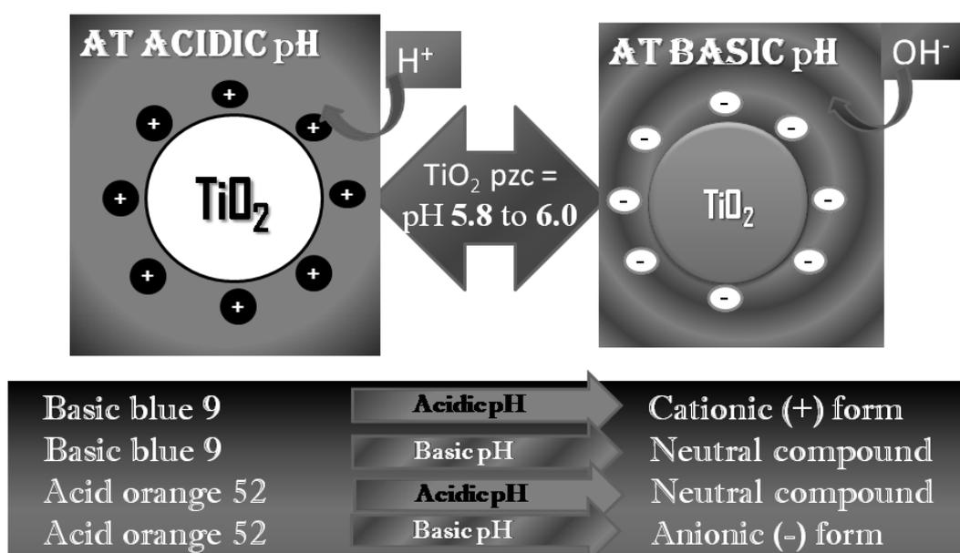
Fig. 6 Dye-Catalyst interaction at acidic pH and basic pH
