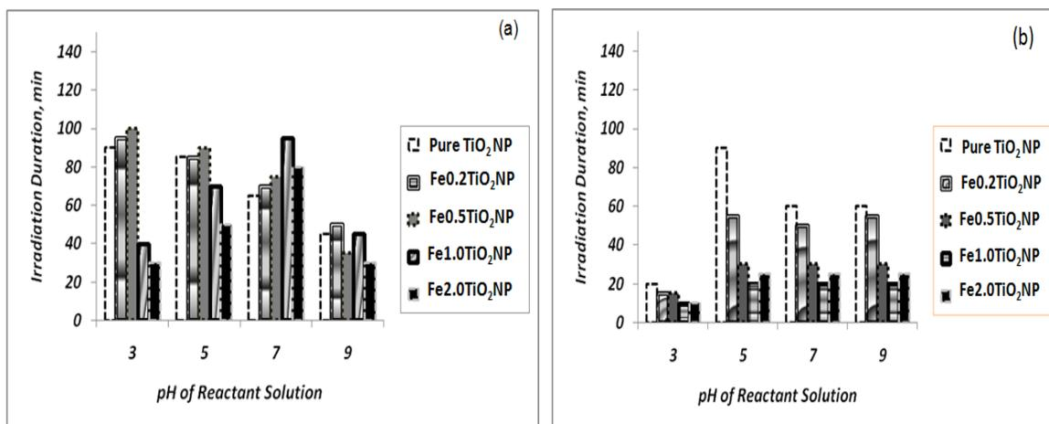
Fig. 5 Coupled semiconductor photo-Fenton's decolorization of (a) BB dye and (b) AO dye with pure and Fe-TiO<sub>2</sub> nanotitania at varied pH (Experimental conditions: Catalyst dosage=0.5 g/L; H<sub>2</sub>O<sub>2</sub> concentration=29.7 mmol/L; Initial solar intensity during BB decolorization= $\sim$ 60kiloLUX; Initial solar intensity during AO decolorization= $\gt$ 90kiloLUX)
