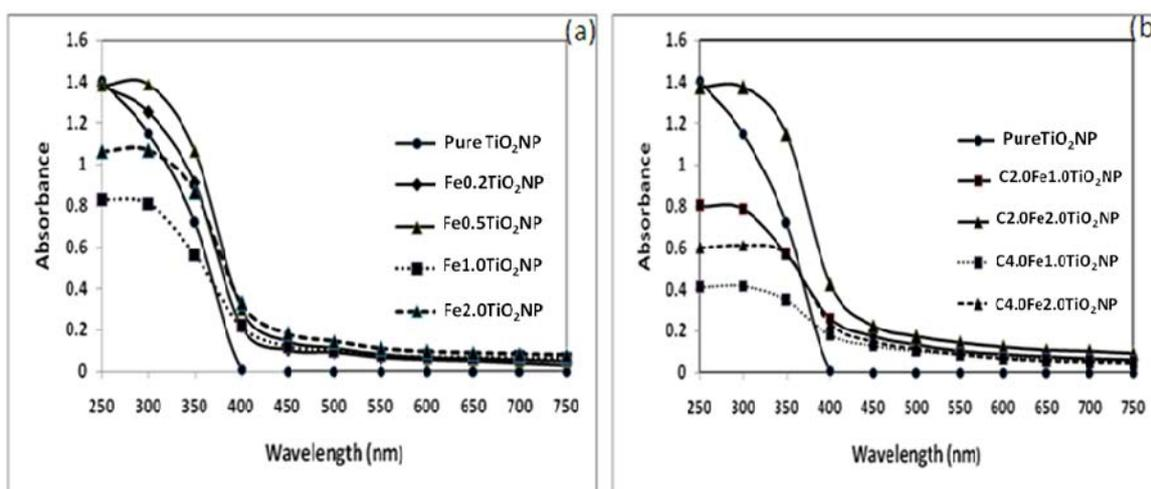
Fig. 4 UV-Vis Absorption Spectra of (a) pure and iron doped catalysts (b) pure and carbon-iron codoped catalysts
