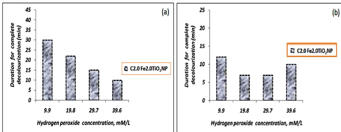
Fig 9. Effect of hydrogen peroxide concentration in the decolorization of (a) BB(b) AO dye (Experimental conditions : Initial concentration of dye = 10 ppm; Catalyst dosage = 0.75 g/L (for BB), 1.0 g/L (for AO); Initial solar intensity ~60,000 LUX)
