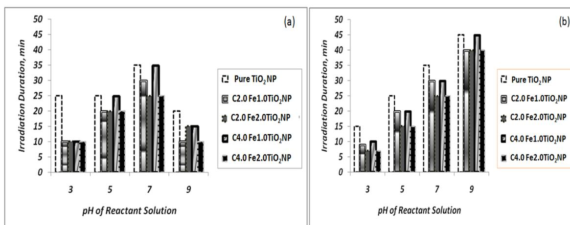
Fig. 7 Coupled semiconductor photo-Fenton's decolorization of (a) BB (b) AO with pure and C-Fe codoped nanotitania at varied pH (Initial solar intensity (BB) = ~55 kiloLUX; Initial solar intensity (AO) = ~50 kiloLUX)
