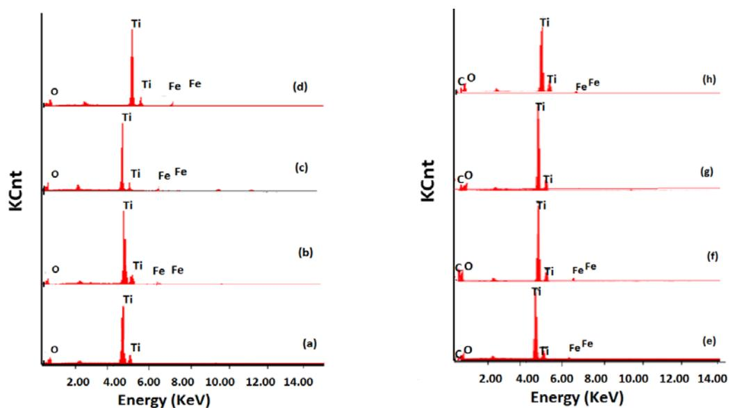
Fig. 3 EDX spectra of (a)  $\text{Fe}_{0.2}\text{TiO}_2\text{NP}$  (b)  $\text{Fe}_{0.5}\text{TiO}_2\text{NP}$  (c)  $\text{Fe}_{1.0}\text{TiO}_2\text{NP}$  (d)  $\text{Fe}_{2.0}\text{TiO}_2\text{NP}$  (e)  $\text{C}_{2.0}\text{Fe}_{1.0}\text{TiO}_2\text{NP}$  (f)  $\text{C}_{2.0}\text{Fe}_{2.0}\text{TiO}_2\text{NP}$  (g)  $\text{C}_{4.0}\text{Fe}_{1.0}\text{TiO}_2\text{NP}$  (h)  $\text{C}_{4.0}\text{Fe}_{2.0}\text{TiO}_2\text{NP}$
