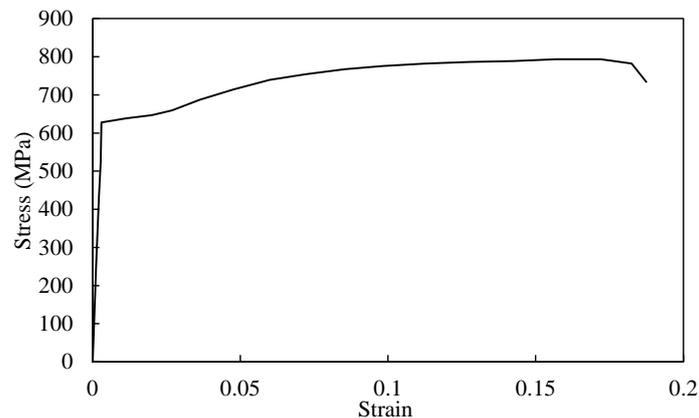
Fig. 5 Measured stress-strain curve of reinforcing bar
