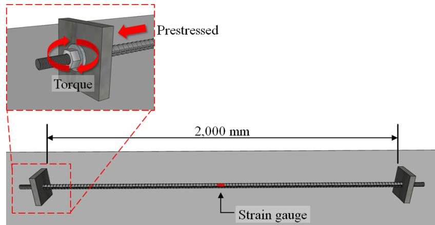
Fig. 4 Schematic of long reinforcing bar with set of washer and nut
