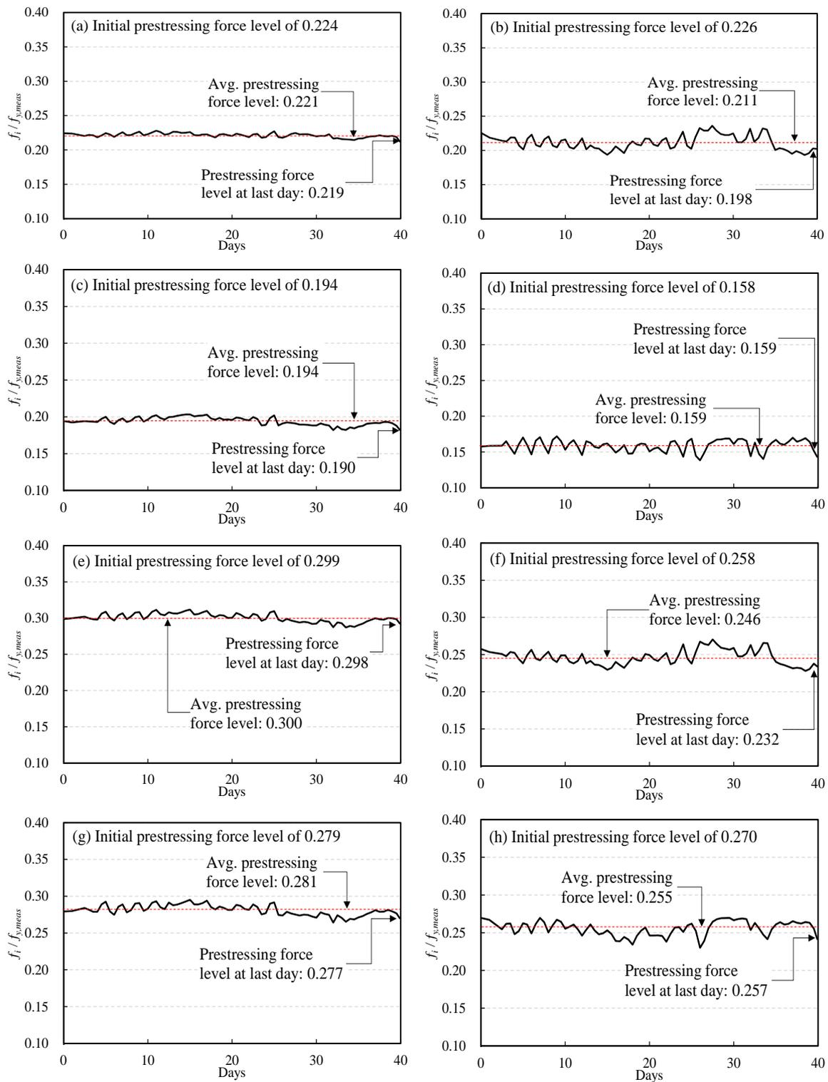
Fig. 7 Relaxation test results (set of flat washer and hex nut)
