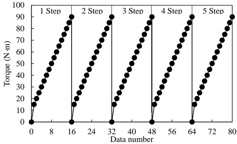
Fig. 2 Loading plan
