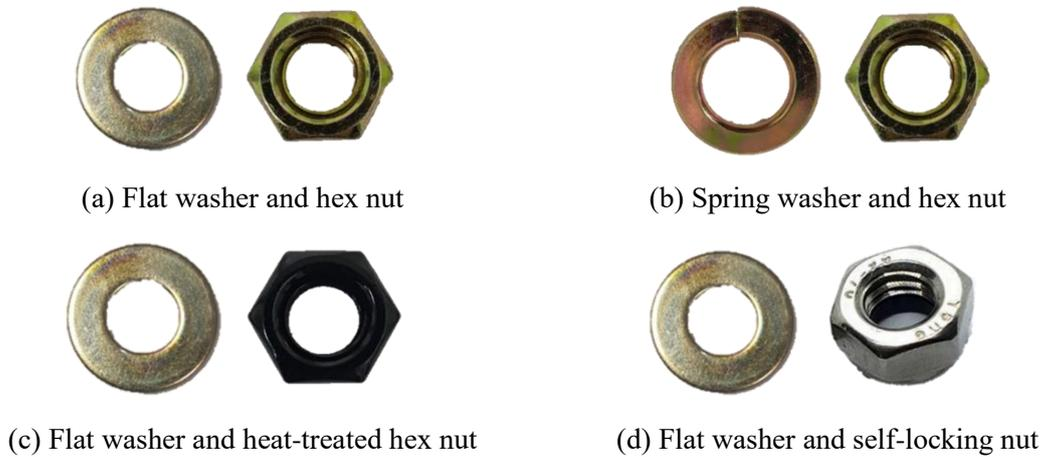
Fig. 1 Sets of washer and nut
