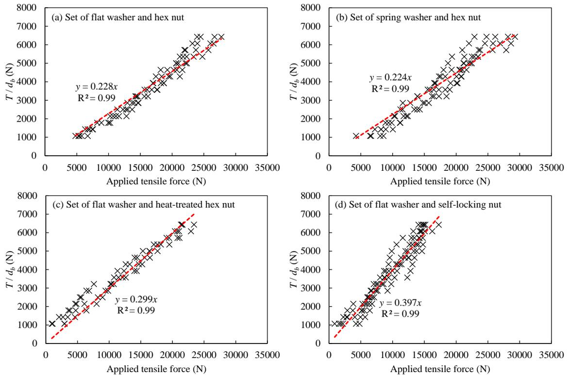
Fig. 6 Relationship between applied tensile force and  $T/d_b$  for each washer–nut set
