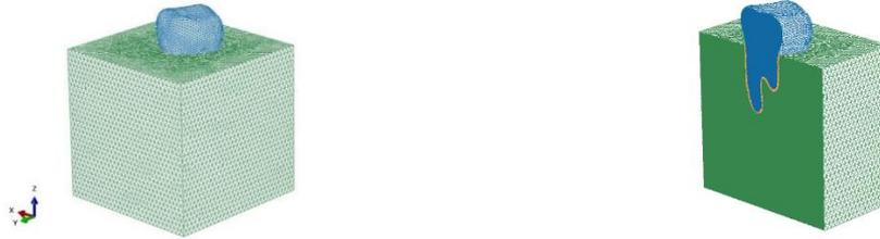
Fig. 1 The proposed single tooth FE model. Left figure shows a single tooth model consisting of tooth #16, PDL, and bone in blue, orange, and green color, respectively. Right figure shows cross section of the model
