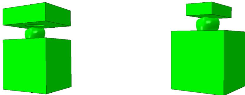
(a) Single tooth model with a cap. To simulate clenching activity, a cap part has a groove to be matched with the occlusal surface of the tooth part
