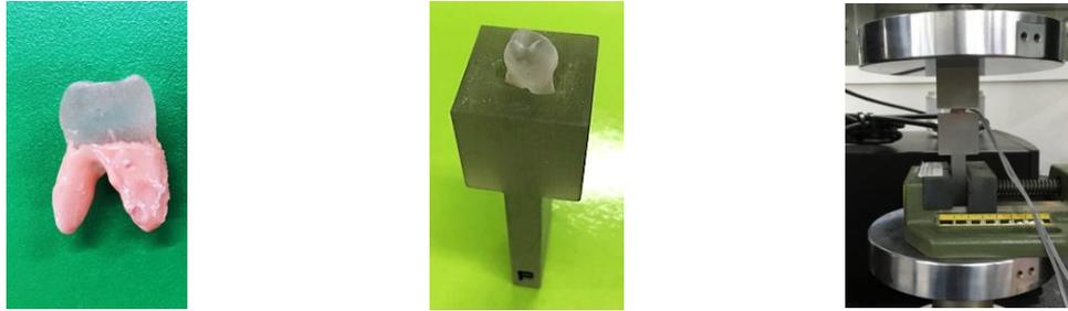
(a) Tooth specimen applied with the silicone impression for the PDL (b) Tooth installed into the bone cube (c) Test setup. The bone cube was clamped to test-zig
