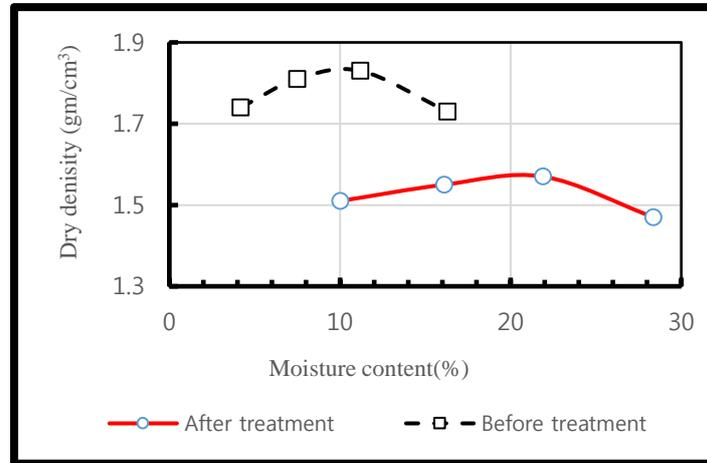
Fig.4 Compaction curves Before and After Treatment
