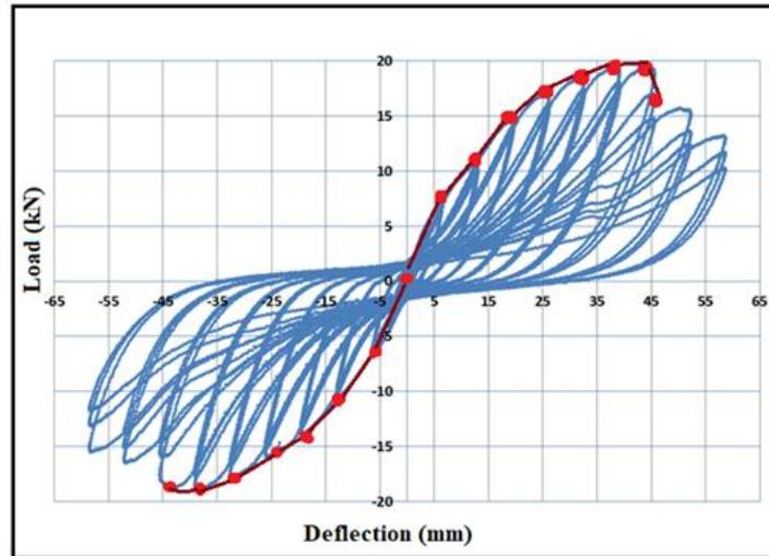
Fig. 4 The typical cyclic test result for Series 2, Test 1C: 12.7 mm (½ in.) SIS
