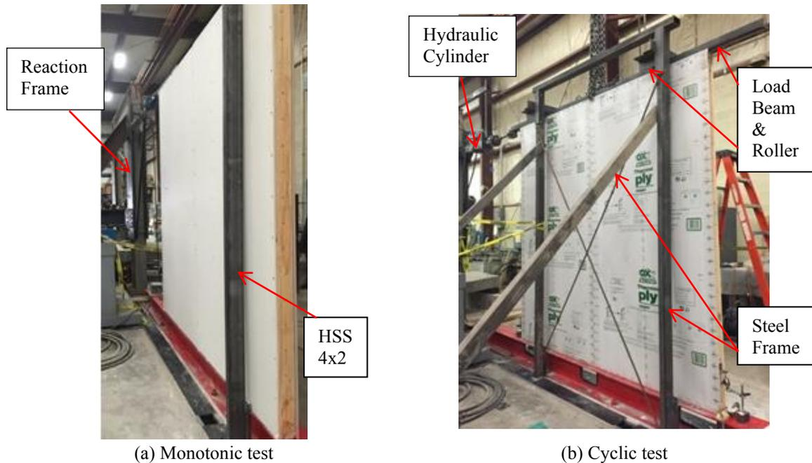
Fig. 2 Frame used to control out-of-plane deformation
