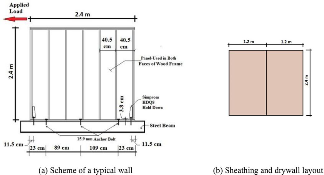
Fig. 1 Typical test wall configuration
