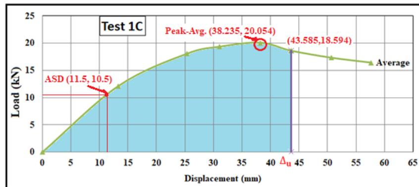
Fig. 6 Typical average envelope curve (Test 1C) used to determine ultimate displacement
