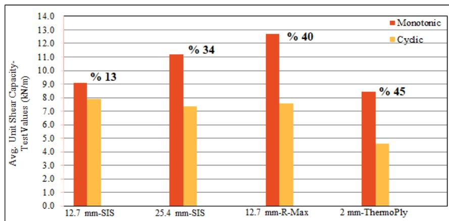
Fig. 3 Test results for monotonic tests in comparison to the cyclic tests
