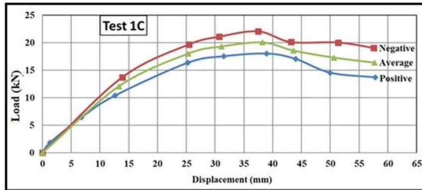
Fig. 5 The typical cyclic test result for Series 2, Test 1C: 12.7 mm (½ in.) SIS
