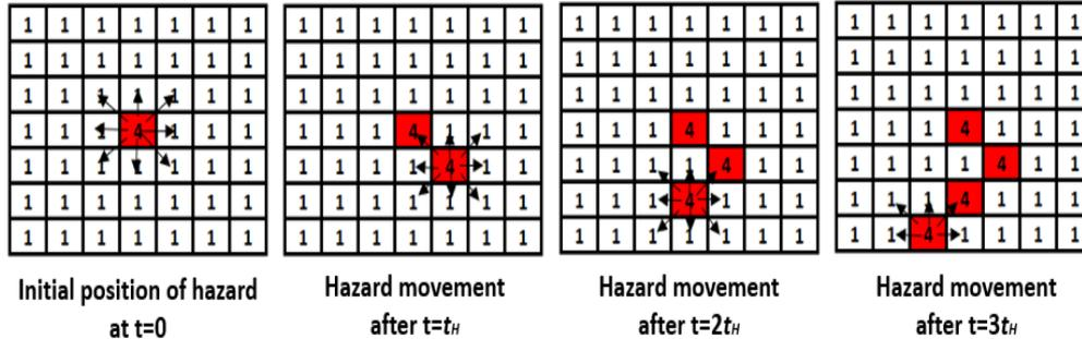
Fig. 7 Schematic representation of random hazard movement in EVAQ
