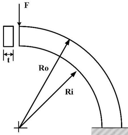
Fig. 4 Curved cantilever beam
