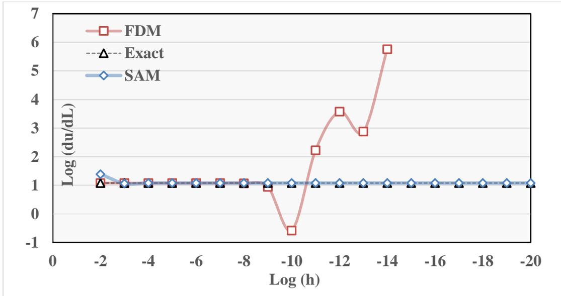
Fig. 3 Vertical displacement sensitivity of the beam tips for square elements
