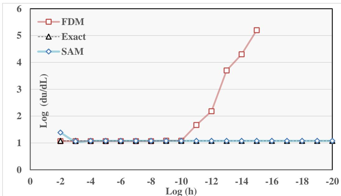
Fig. 2 Vertical displacement sensitivity of the beam tips for triangular elements
