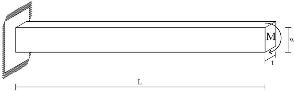
Fig. 1 Cantilever beam with the rectangular section
