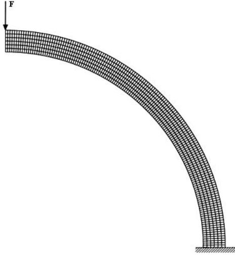
Fig. 5 Meshing of the curved cantilever beam
