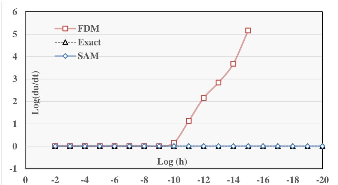
Fig. 7 Horizontal displacement sensitivity respect to the beam thickness
