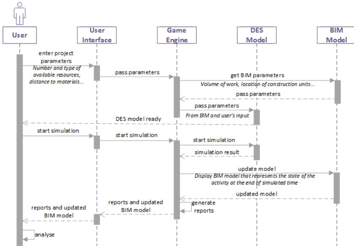
Fig. 2 Prototype sequence diagram
