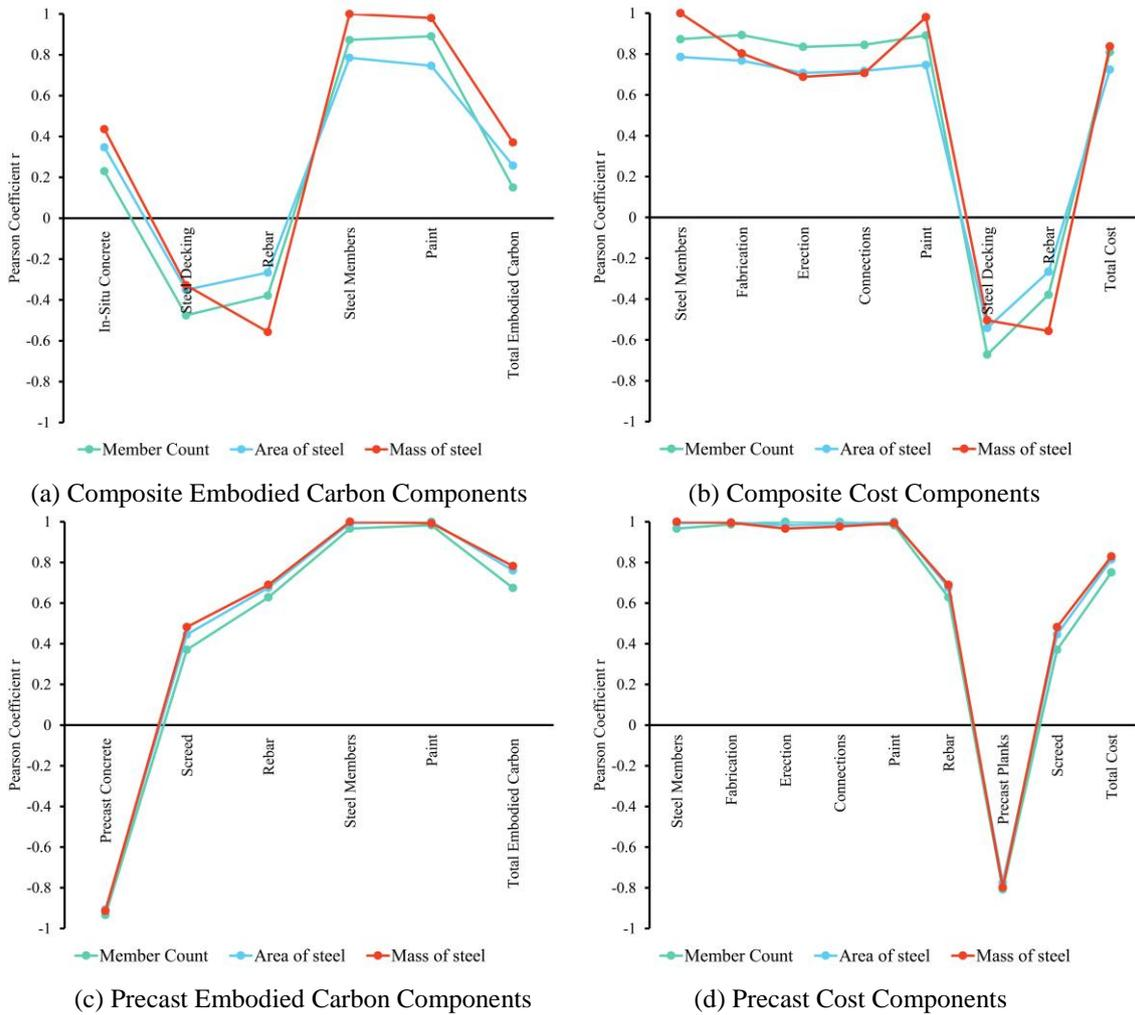
Fig. 7 Correlation between the steel member count, area of steel and steel weight with the cost and carbon performance of the 29 designs
