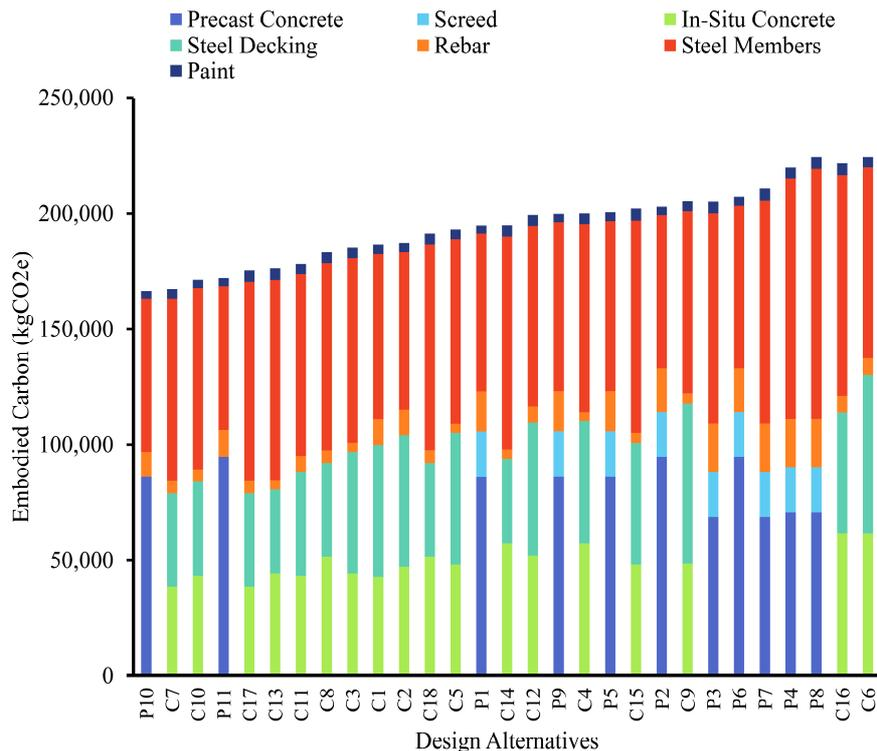
Fig. 4 Embodied carbon performance of the 29 designs generated by engineering practitioners
