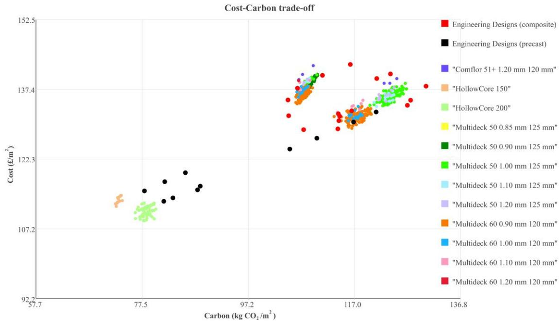
Fig. 9 The solution space for the tested building case with the optimised solutions from the structural engineers and the automated design analyses
