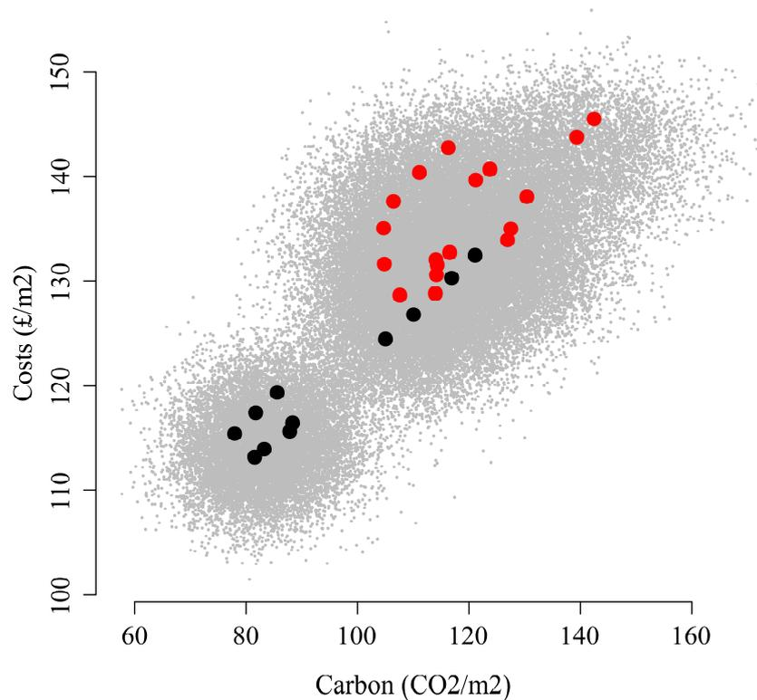
Fig. 8 Uncertainty analysis for the 29 design configurations. The composite designs are shown with the red nodes and the precast designs with black nodes.
