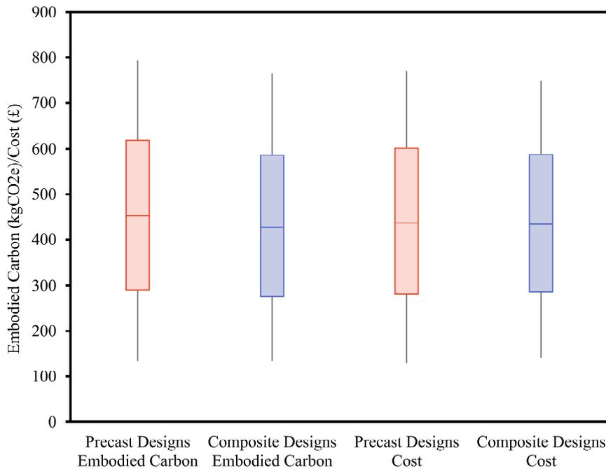
Fig. 6 Box plots showing the overall cost and embodied carbon performance per m2 of floor are for the composite and precast designs implementing the minimum, the 1st quartile, the median, the 3rd quartile and the maximum values from the entire solution set
