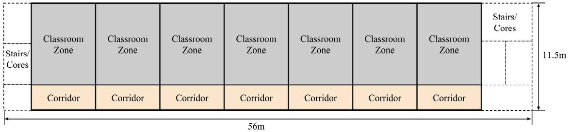
Fig. 2 Typical floor layout of the tested building case
