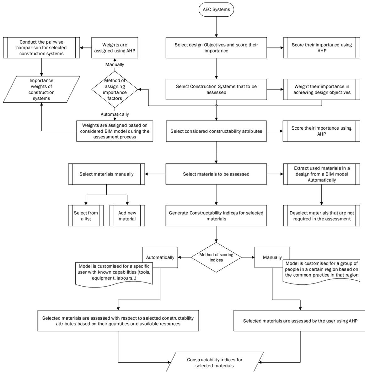
Fig. 4 Customising AEC systems in constructability assessment model
