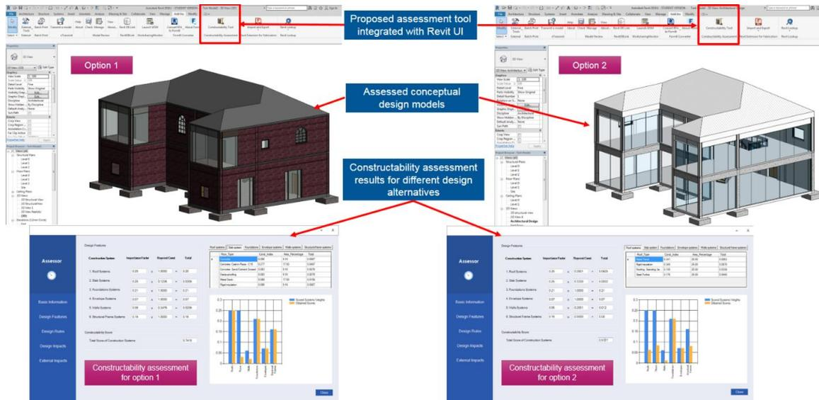
Fig. 8 Constructability scores of design alternatives
