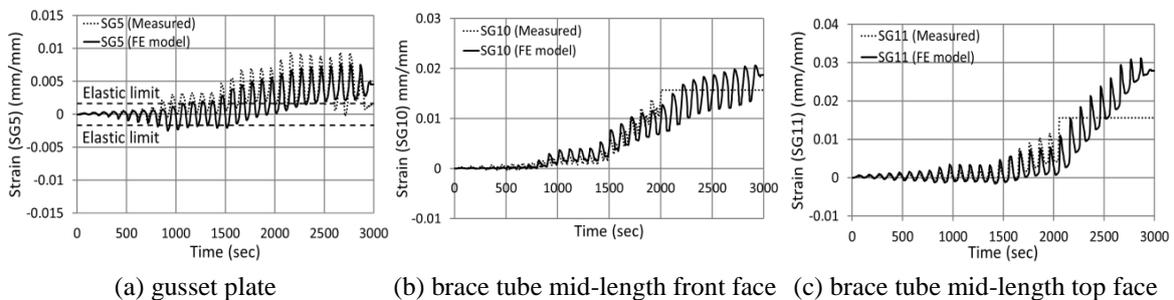
Fig. 22 Plots of strain recording versus time magnitude obtained from FE and test models for specimen of S40-CA-G2-2 at various locations, as identified in Fig. 18
