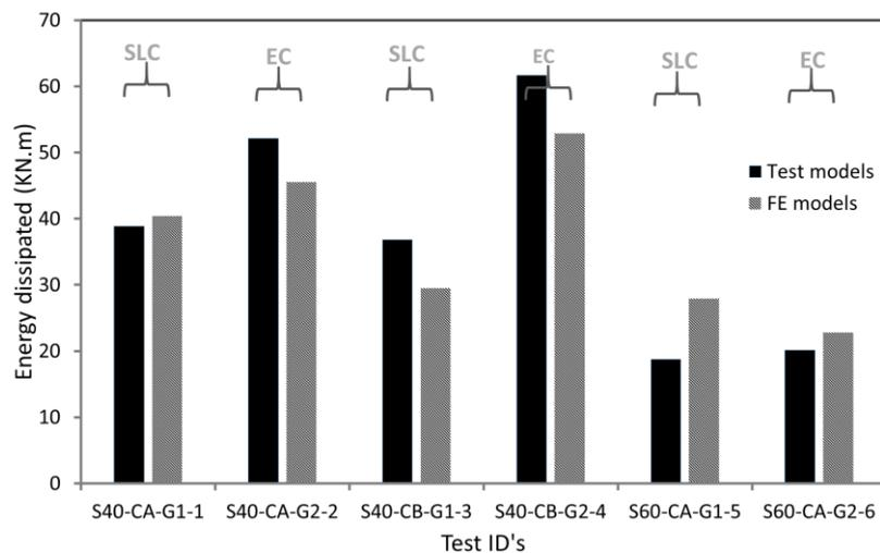
Fig. 25 Energy dissipation capacity of the physical test models and FE models
