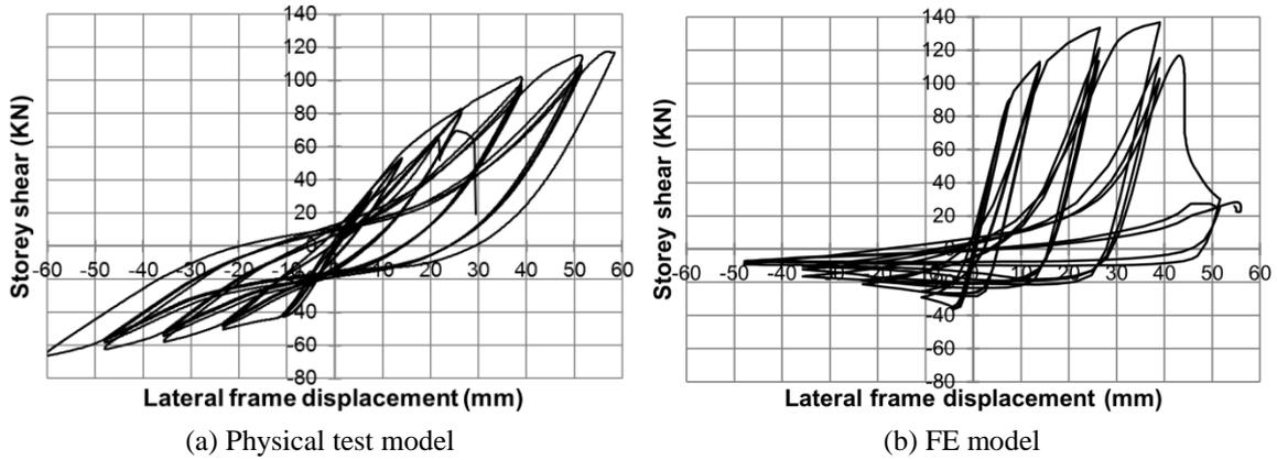
Fig. 8 Plots of storey shear versus lateral frame displacement of specimen S40-CA-G1-1.
