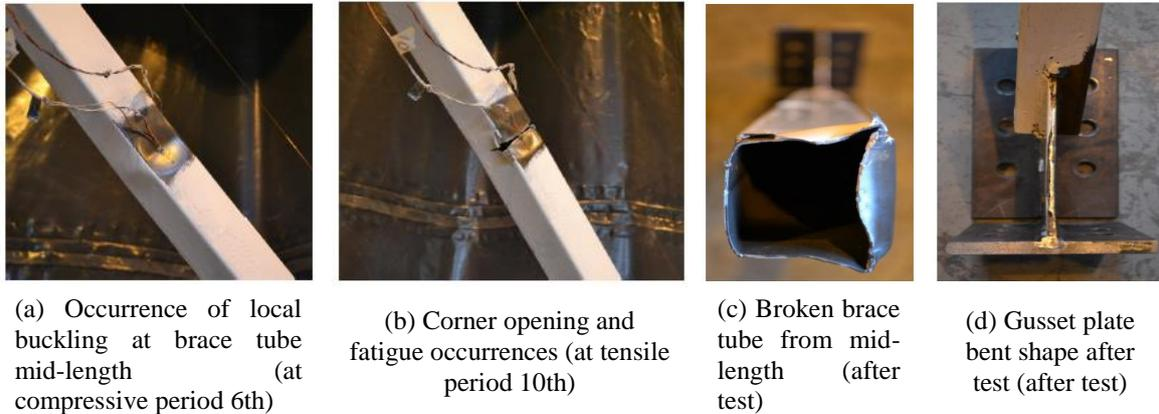
Fig. 26 Snapshots of specimen S60-CA-G1-5 during testing programme
