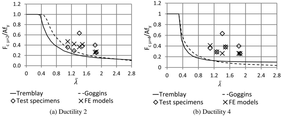
Fig. 15 Plots of normalised post-buckling loads versus normalised slenderness ratio, including predictions from Tremblay (2002) and Goggins (2004)
