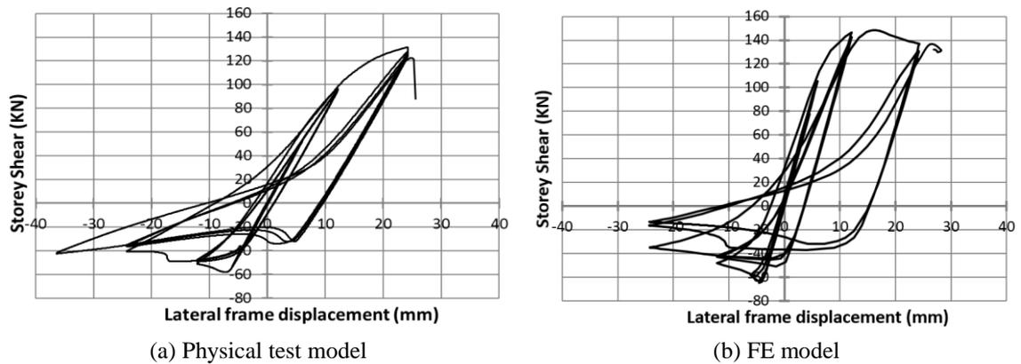
Fig. 13 Plots of storey shear versus lateral frame displacement of specimen S60-CA-G2-6
