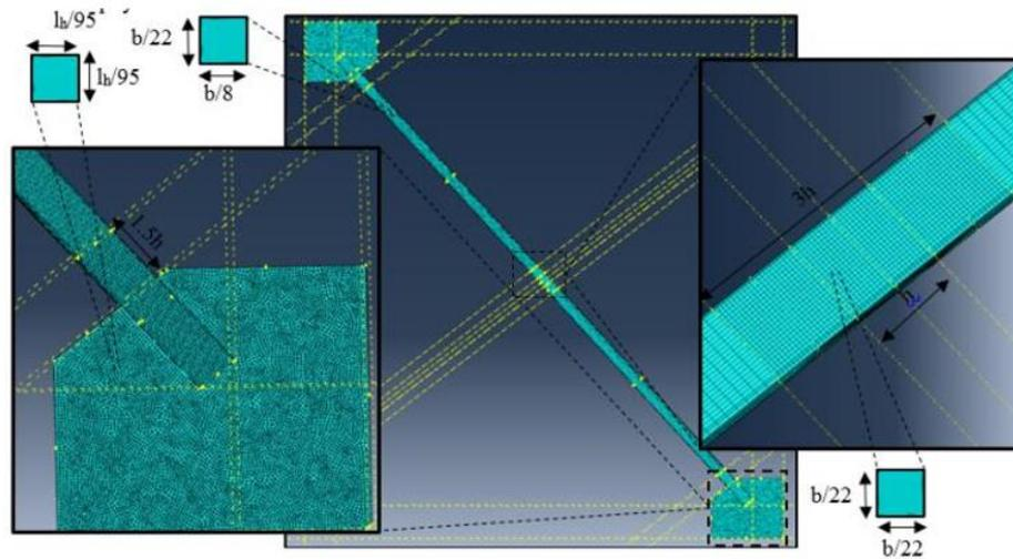
Fig. 7 FE model of S40-CA-G1-1 specimen with mesh detailing in measuring unit (mm)
