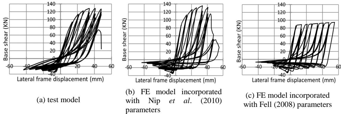
Fig. 5 Plots of base shear versus lateral frame displacement
