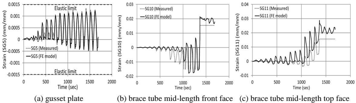
Fig. 21 Plots of strain recording versus time magnitude obtained from FE and test models for specimen of S40-CA-G1-1 at various locations, as identified in Fig. 18
