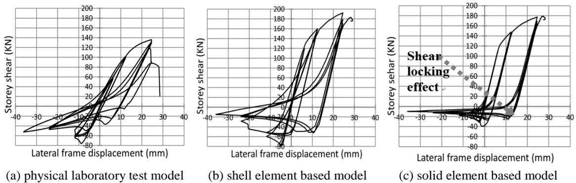
Fig. 6 Plots of base shear versus lateral frame displacement for specimen S60-CA-G1-5
