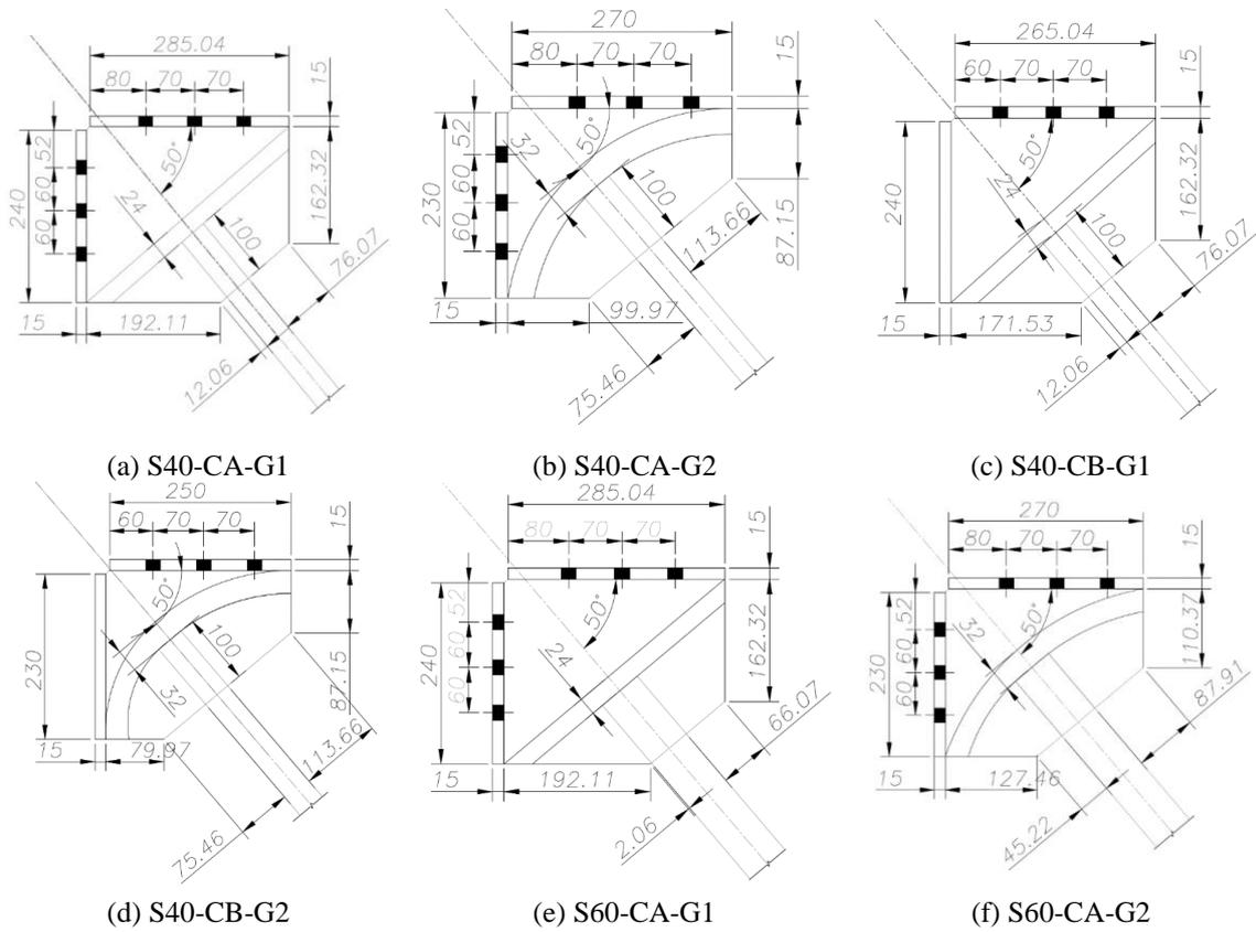
Fig. 1 Detailing of gusset plates in test models
