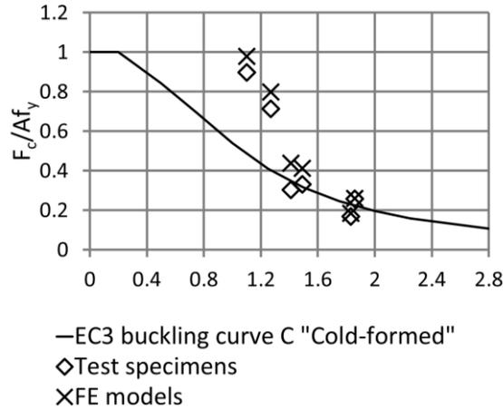
Fig. 14 Plot of normalised initial-buckling loads versus normalised global slenderness ratios for all specimens, including buckling curve from EC3 (CEN 1993)
