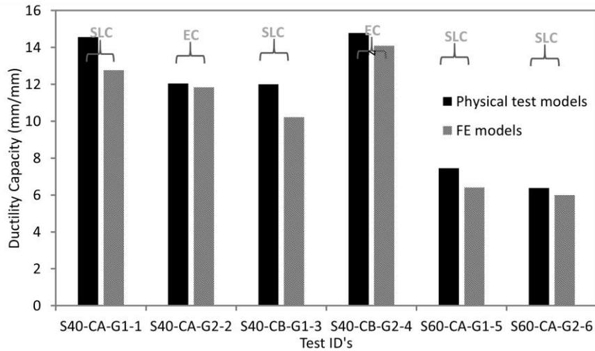
Fig. 24 Ductility capacity of the physical test models and FE models
