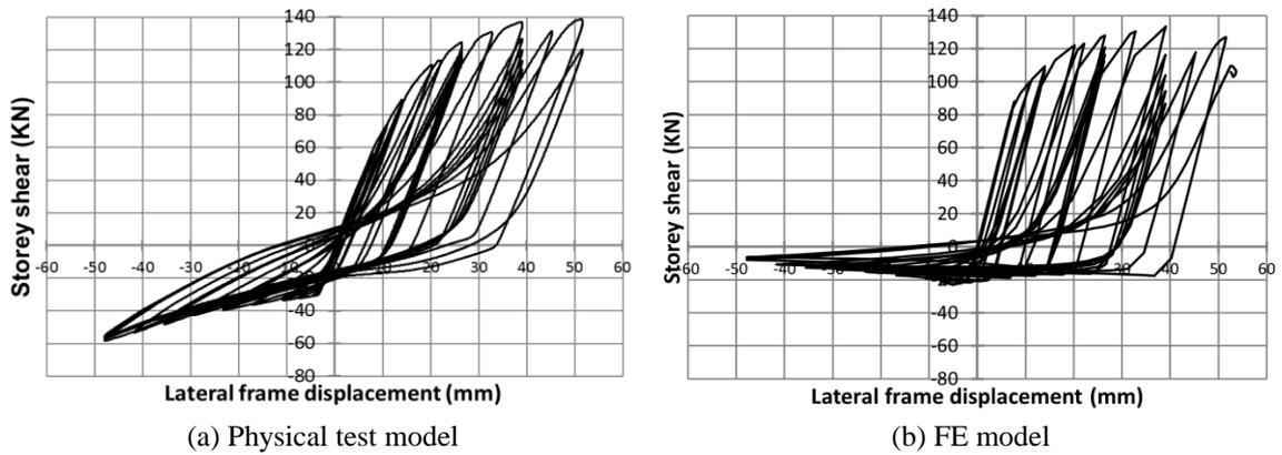
Fig. 9 Plots of storey shear versus lateral frame displacement of specimen S40-CA-G2-2.
