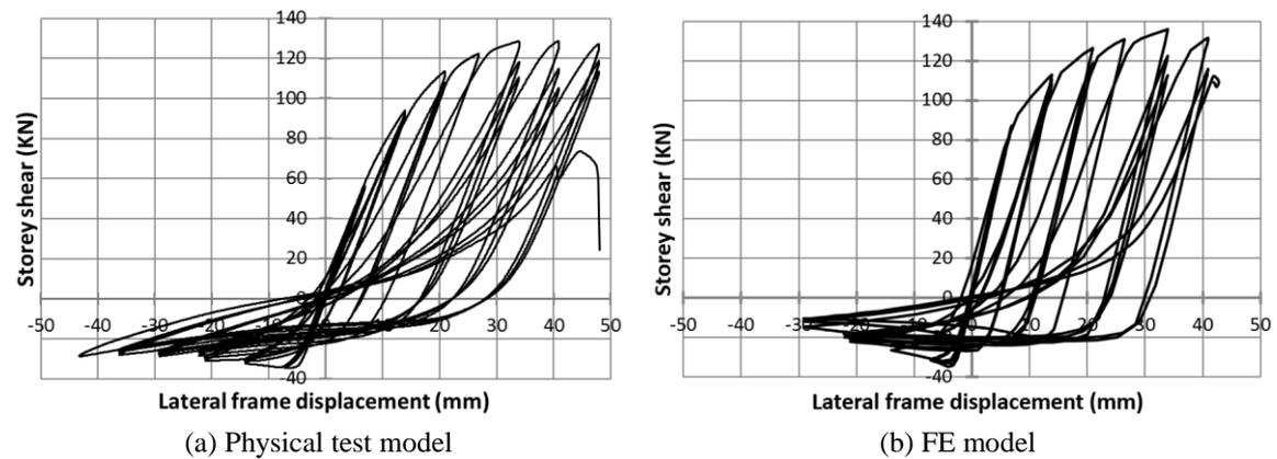
Fig. 10 Plots of storey shear versus lateral frame displacement of specimen S40-CB-G1-3.
