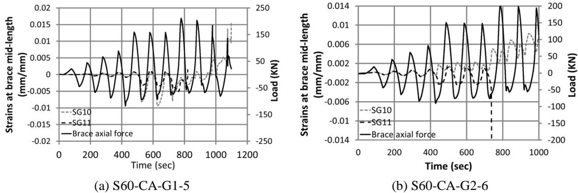
Fig. 19 Plots of measured time-varying longitudinal strains and brace axial force for physical test specimens
