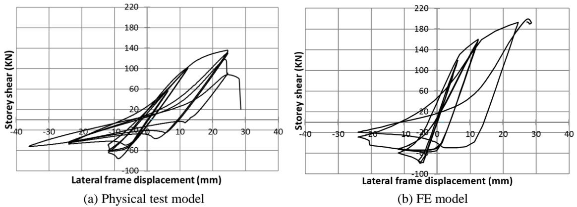
Fig. 12 Plots of storey shear versus lateral frame displacement of specimen S60-CA-G1-5
