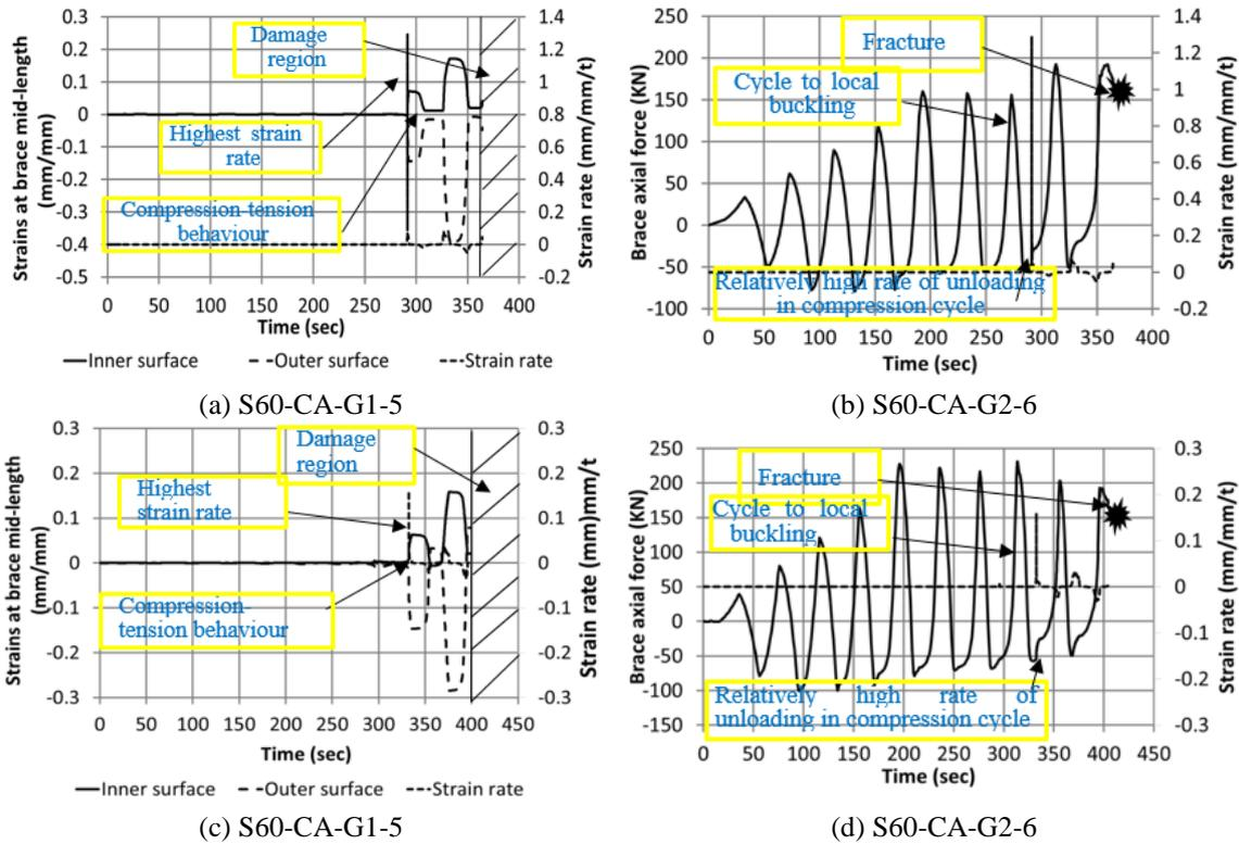
Fig. 20 Plots of (a-b) time-varying longitudinal strain (primary) and strain rate (secondary) from FE models and (c-d) plots of time-varying brace axial force (primary) and strain rate (secondary) from FE models
