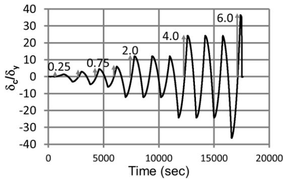
Fig. 3 Profile of loading protocol in accordance with ECCS (1986) guidelines
