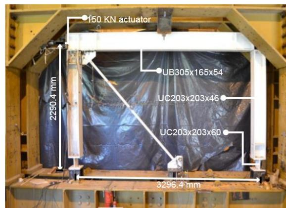
Fig. 2 Test set-up, including frame details
