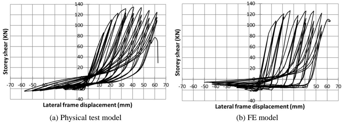
Fig. 11 Plots of storey shear versus lateral frame displacement of specimen S40-CB-G2-4
