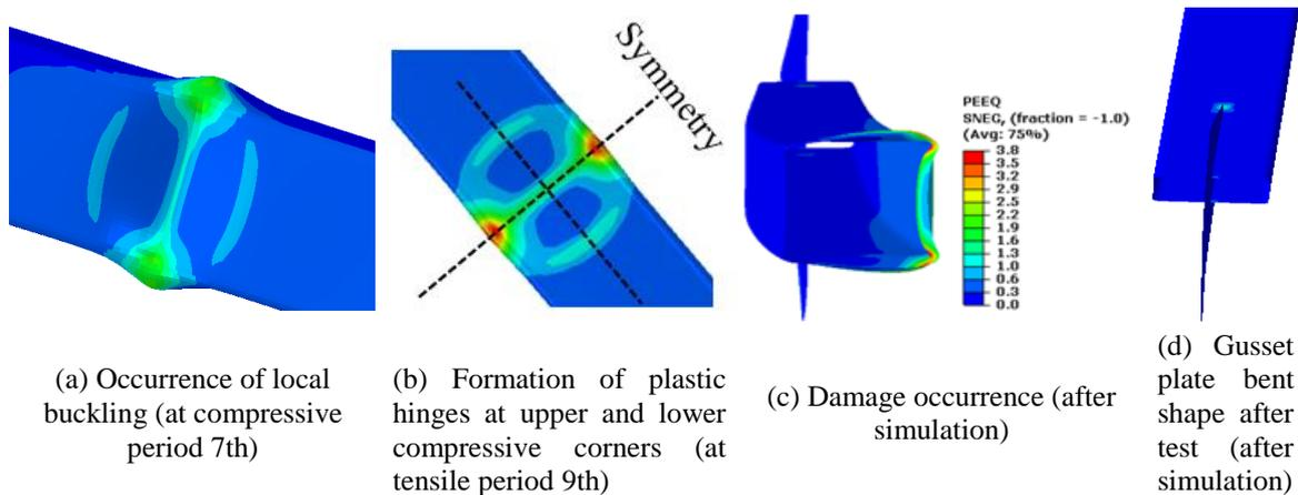
Fig. 27 Snapshots of FE model S60-CA-G1-5 during and after simulation
