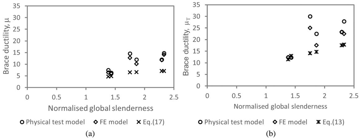
Fig. 23 Comparison of observed peak displacement ductility demand in test to predicted brace ductility capacity in FE models, along with predictions of (a) Nip *et al.* (2010) and (b) Tremblay (2002). Note  $\mu = \delta / \delta_y$  for Nip *et al.* (2010) and  $\mu_T = (\delta_{elong} + \delta_{short}) / \delta_y$  for Tremblay (2002)
