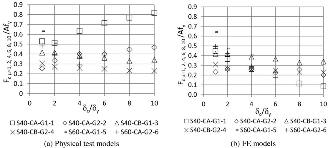
Fig. 16 Post-buckling compressive strength of specimens
