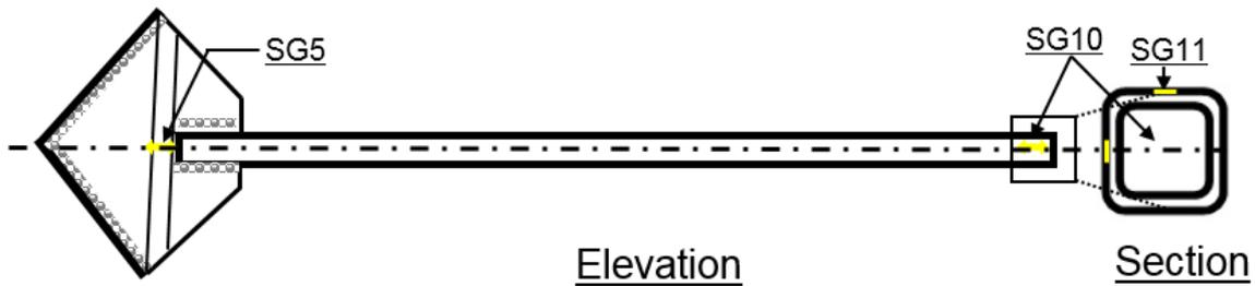
Fig. 18 Location and direction of strain gauges used in the experiments
