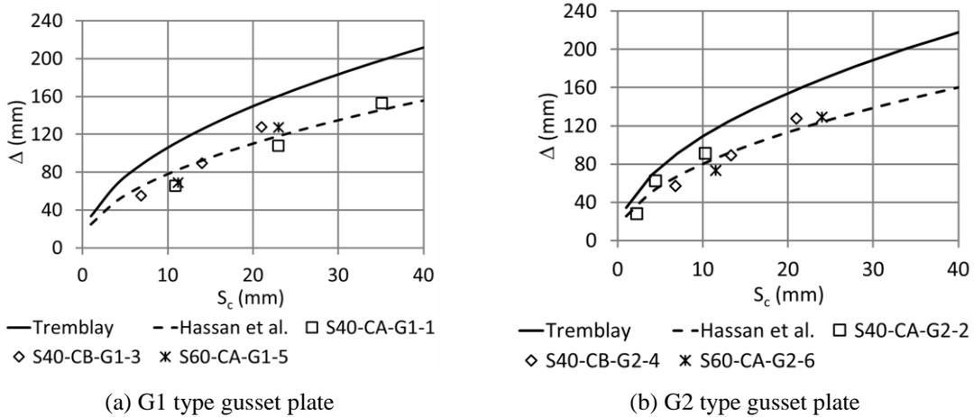
Fig. 17 Plots of lateral deformation of braces against axial displacement magnitude for FE models in conjunction with plots of Tremblay (2002) and Hassan *et al.* (2015).
