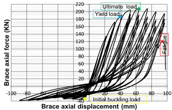
Fig. 4 Plot of hysteresis loops obtained from test model of S40-CB-G2-4 specimen
