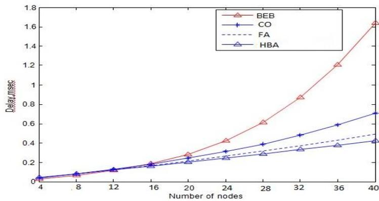
Fig. 5 Nodes vs Transmission delay at different broadcast algorithm
