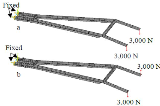
Fig. 3(a) Bending loads and (b) Torsion loads
