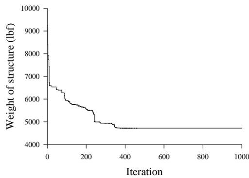
Fig. 7 Weight convergence history for size, shape and topology optimization of the 15-members, 6-nodes truss structure with GSM and iPSO
