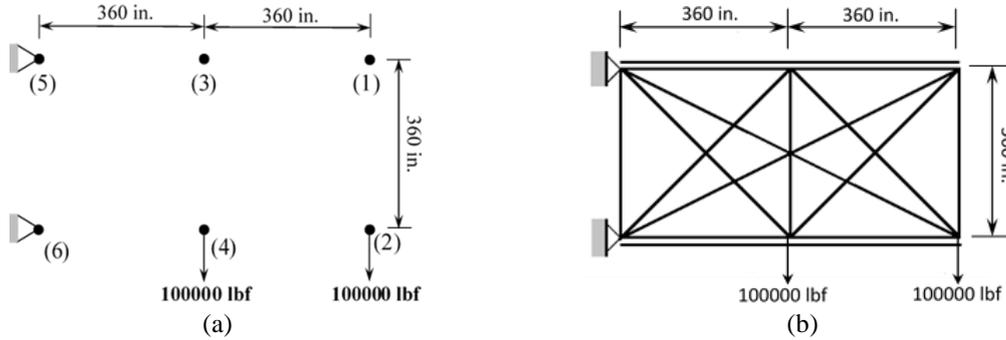
Fig. 5(a) Initial system, (b) Ground structure generated using GSM
