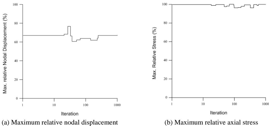
Fig. 17 Relative deflection and stress histories for size, shape and topology optimization of the two-tire planar truss system with TUBM and iPSO
