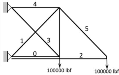
Fig. 6 Optimized structural configuration of the 15-members, 6-nodes truss system found with GSM and iPSO
