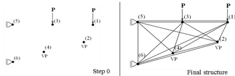
Fig. 1 Creating ground structure using GSM
