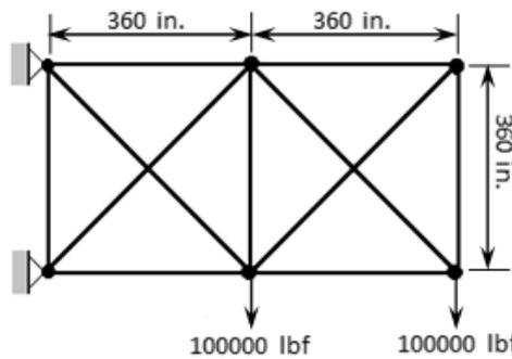
Fig. 9 Ground structure manually generated (Deb and Gulati 2001, Ringertz 1985)
