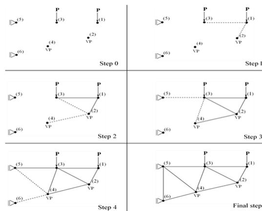
Fig. 2 Creating ground structure using TUBM
