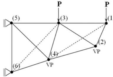
Fig. 3 A sample structure generated by TUBM with two variable points (VPs) and two free elements
