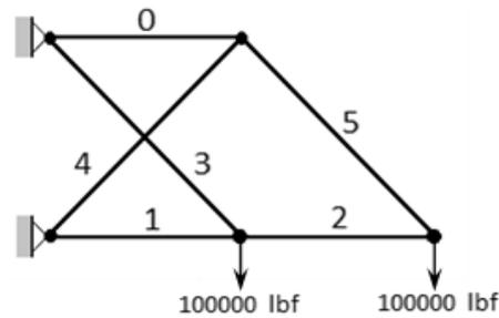
Fig. 10 Optimized structural configuration of the 11-members, 6-nodes truss system found with TUBM and iPSO
