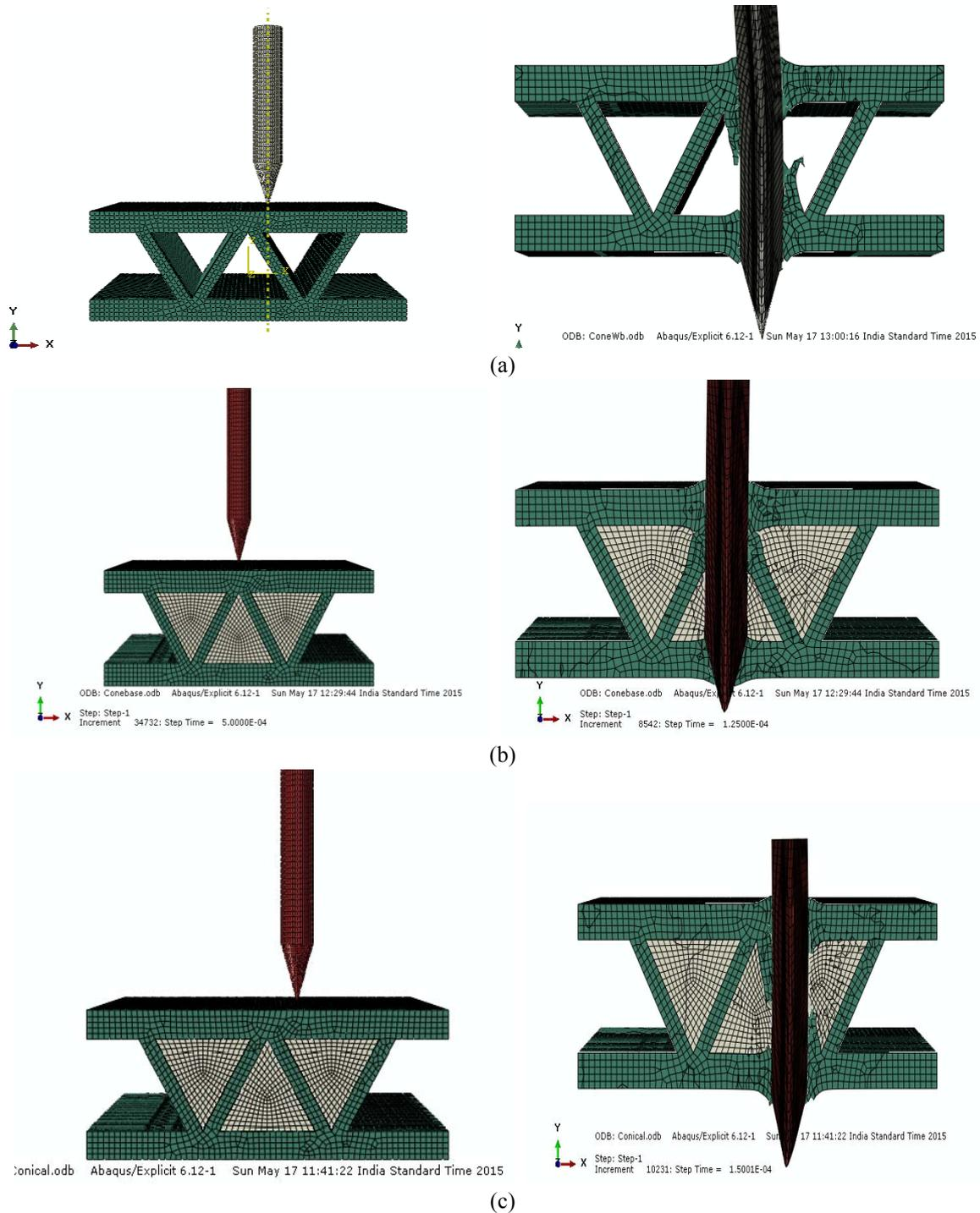
Fig. 4 Comparison of deformed shape of the discretized model (with and without core) due to impact response; (a) Empty corrugated plate web impact, (b) Foam filled corrugated plate base impact and (c) Foam filled corrugated plate web impact
