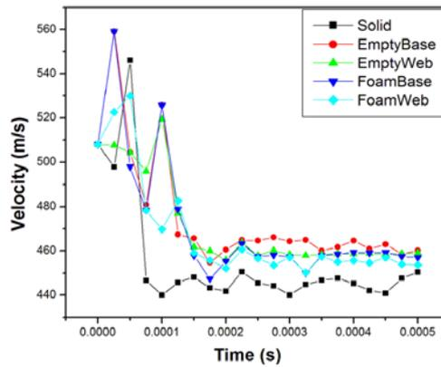
Fig. 11 Velocity-time response for ogive-nose projectile for a varied impact
