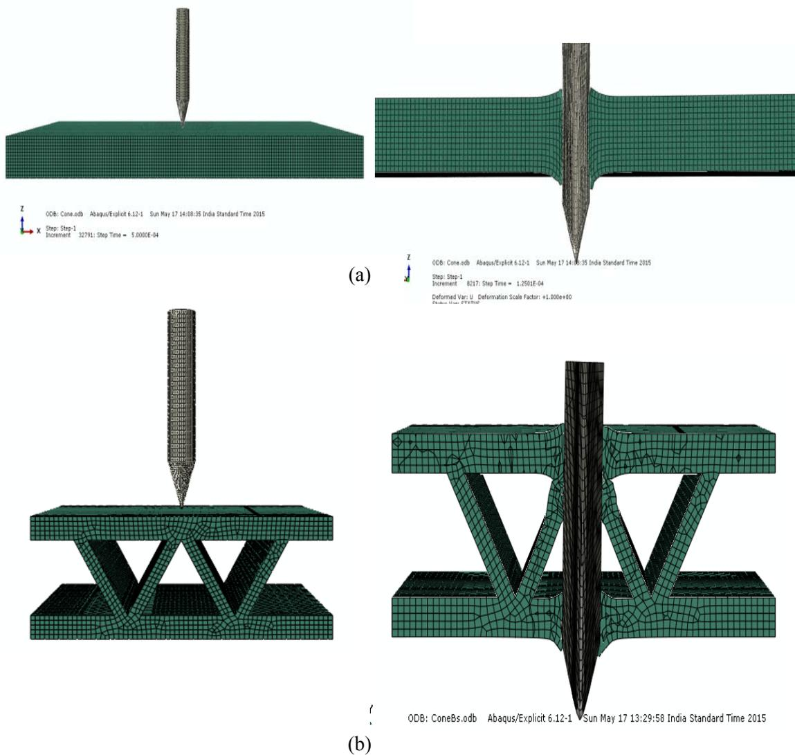
Fig. 3 Deformed shape of the discretized model (without core) due to impact response; (a) Solid plate impact and (b) Empty corrugated plate base impact
