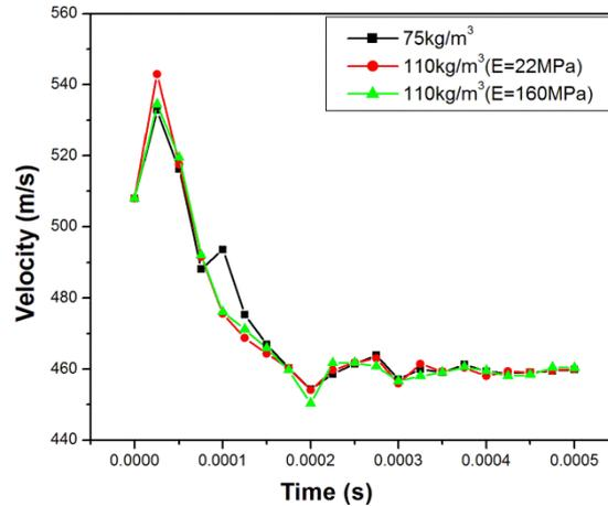
Fig. 7 Velocity-time plot for projectile impacting on PMI foam core corrugated sandwich plate
