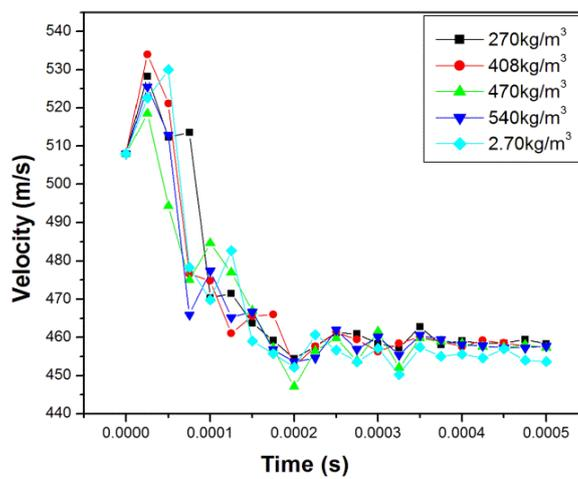
Fig. 6 Velocity-time response for projectile impacting on Aluminum foam core corrugated sandwich plate
