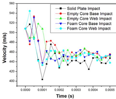
Fig. 12 Velocity-time response for conical-nose projectile for a varied impact
