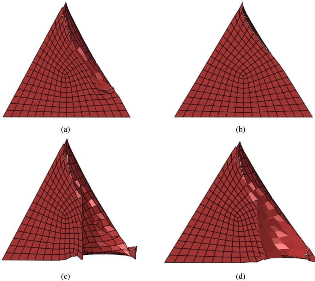
Fig. 5 Foam failure on web impact at different time interval; (a)  $25\mu s$ , (b)  $75\mu s$ , (c)  $150\mu s$  and (d)  $200\mu s$
