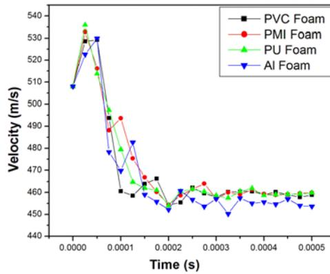
Fig. 10 Comparison of velocity-time response for projectile impacting on different foam core corrugated sandwich plate
