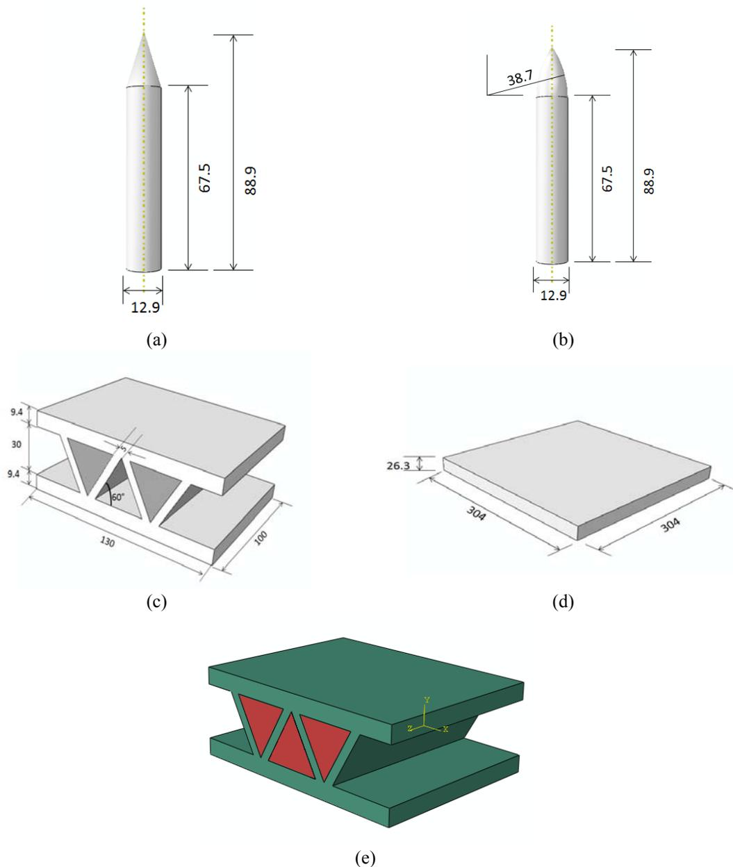
Fig. 1 Physical model along with the dimensions; (a) Conical nose projectile, (b) Ogive nose projectile, (c) Solid target, (d) Empty corrugated target and (e) Foam filled corrugated target (All dimensions are in mm)
