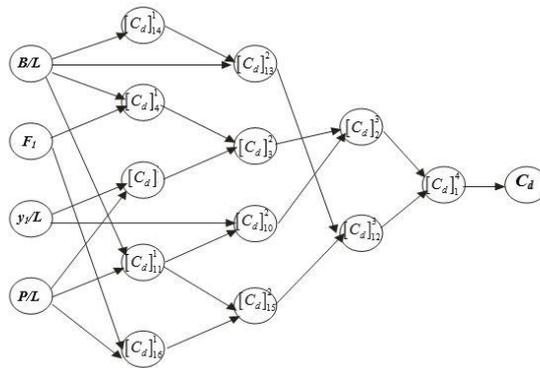
Fig. 8 Network Architecture of the GMDH model for predicting the coefficient of discharge
