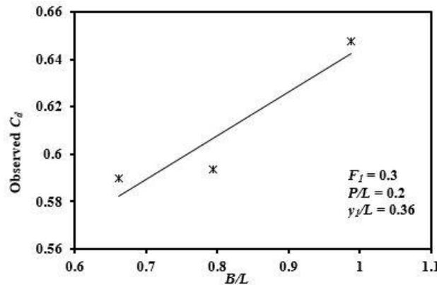
Fig. 4 Variation of  $C_d$  with  $B/L$
