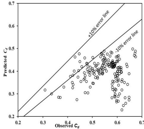
Fig. 5 Comparison between observed and predicted  $C_d$  for Bhorghei *et al.* (1999) model for all data sets
