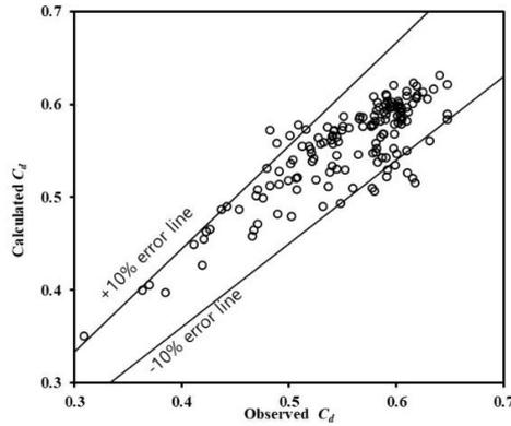
Fig. 7 Comparison between observed and predicted  $C_d$  for Shariq *et al.* (2018) model for all data sets
