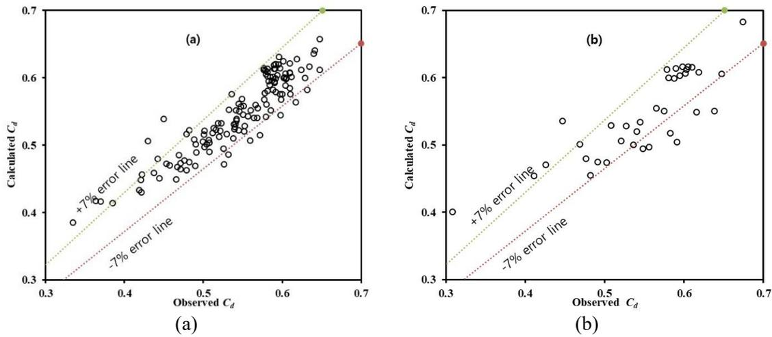
Fig. 12(a) Comparison between predicted and observed  $C_d$  using present GEP model for training data sets
