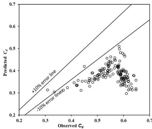
Fig. 6 Comparison between observed and predicted  $C_d$  for Ghodsian (1997) model for all data sets
