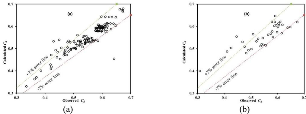
Fig. 9 Comparison between predicted and observed  $C_d$  using present GMDH model for training data sets
