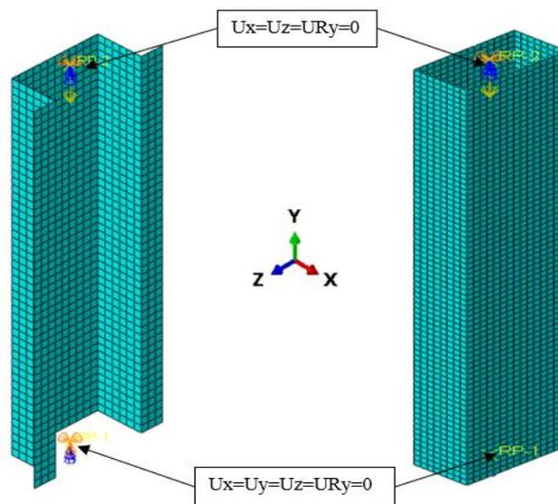
Fig. 4 Applied boundary conditions with open and closed cross-section
