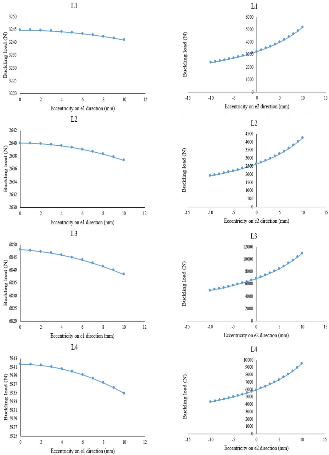
Fig. 6 load eccentricity versus buckling load - C1 section
