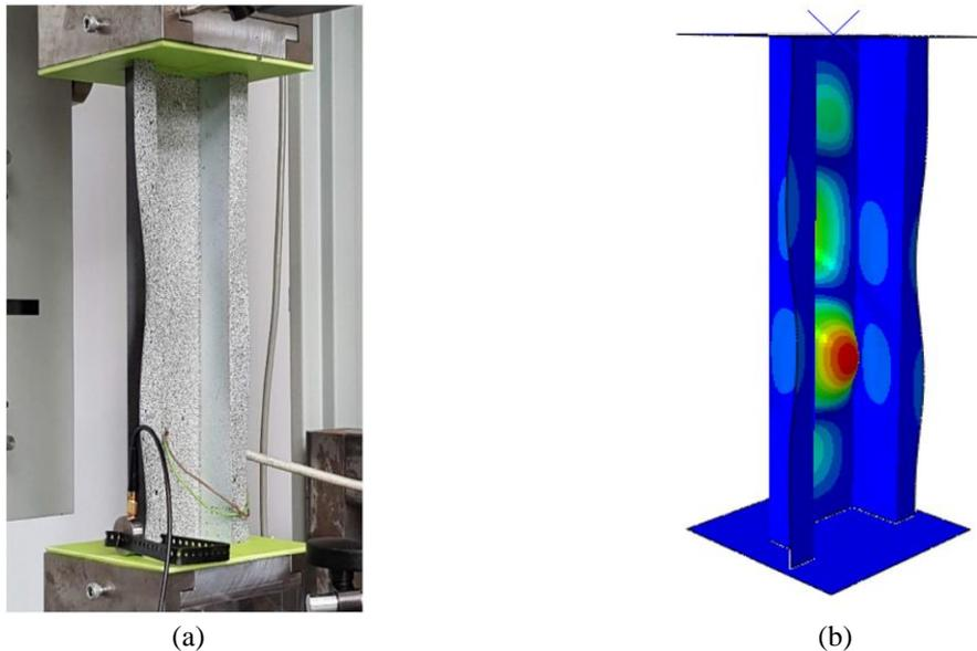
Fig. 5 Buckling mode of structure under axial compression: a) experimental, b) numerical.
