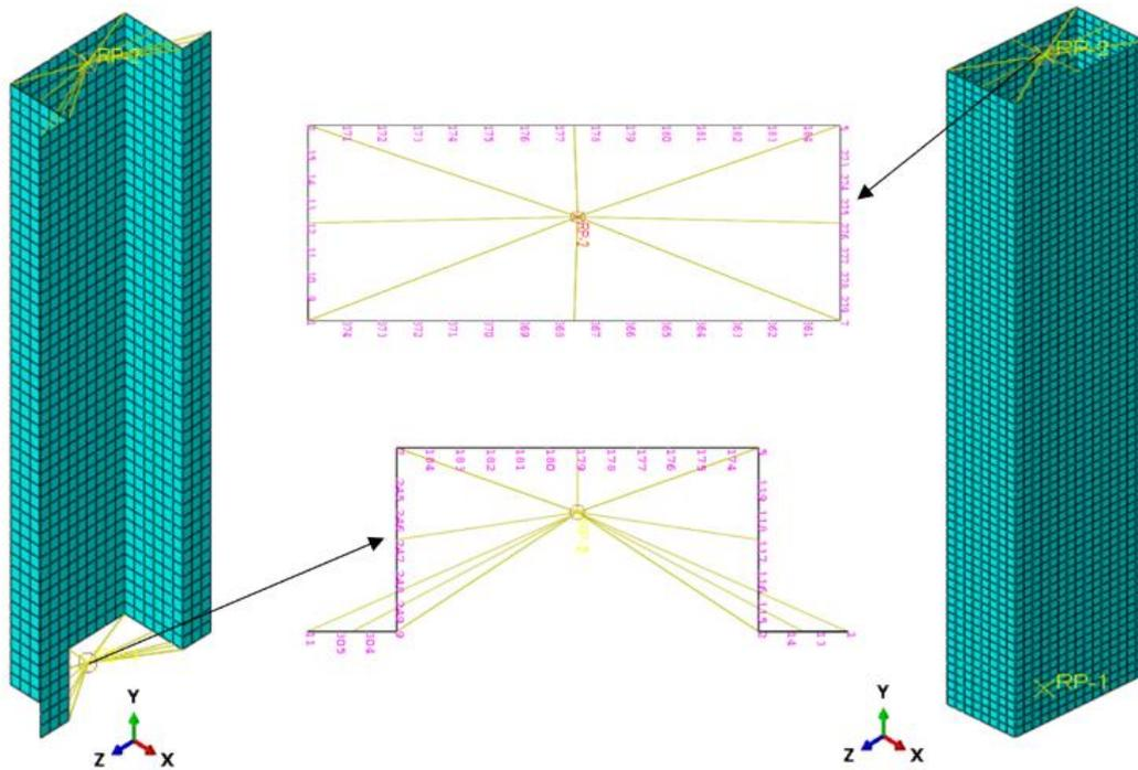
Fig. 2 Discrete model of column with open and closed cross-section
