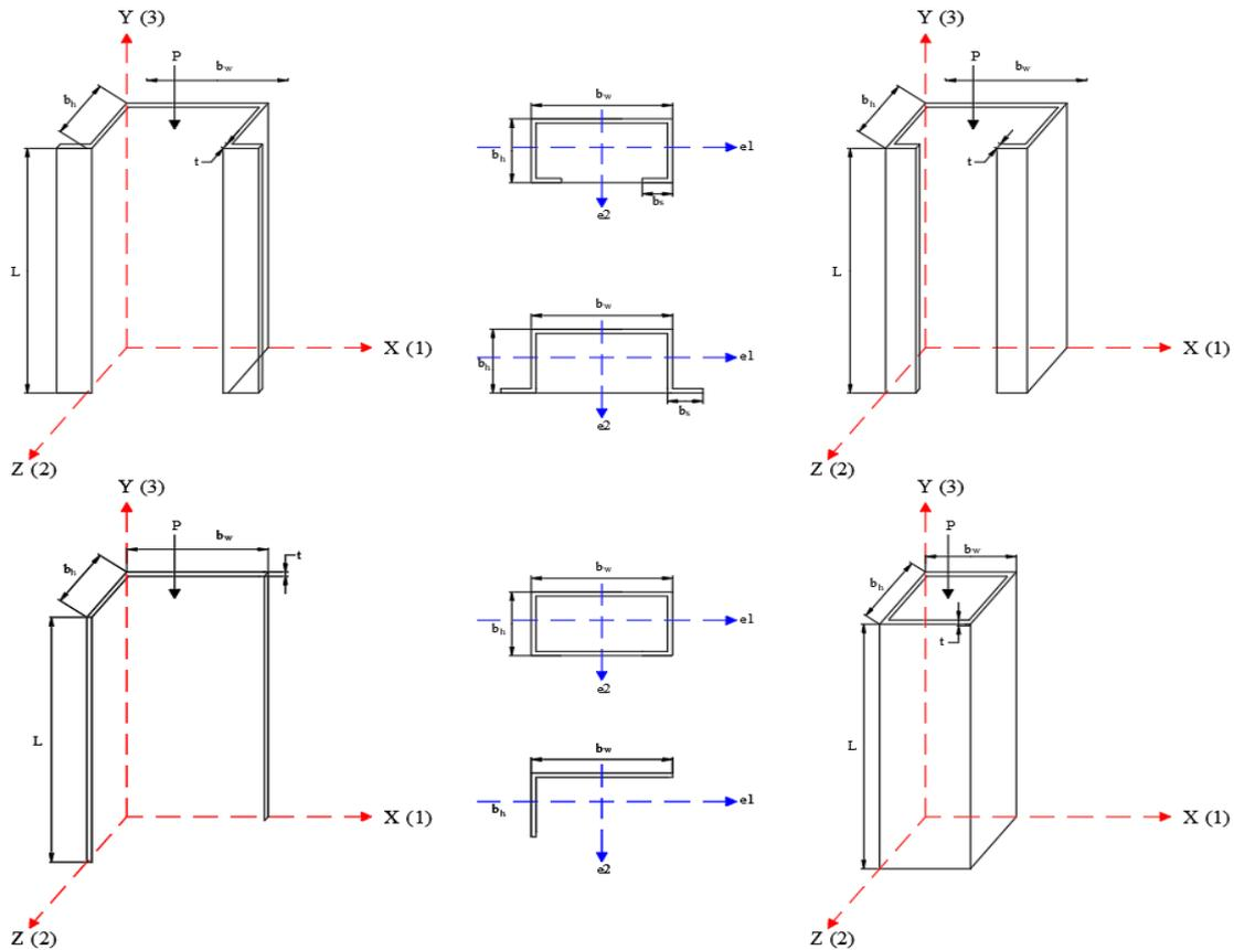
Fig. 1 Cross-section notations of PFRP column profiles
