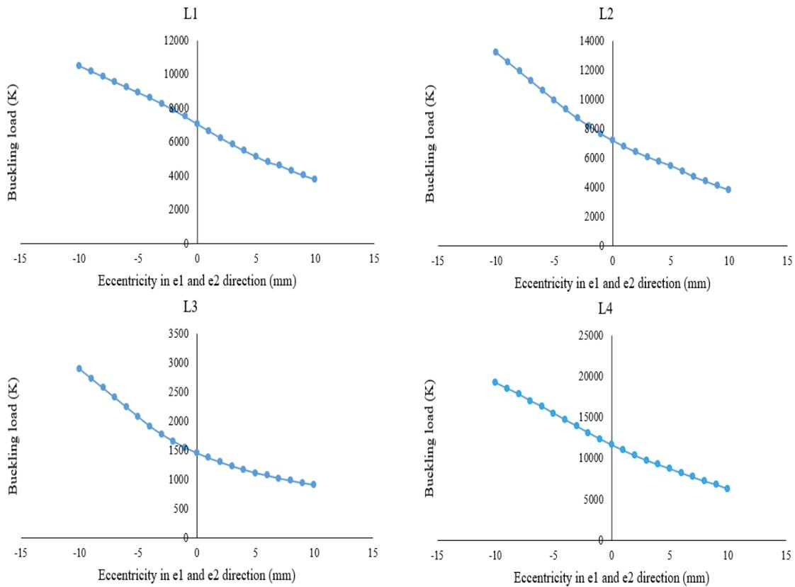
Fig. 9 Load eccentricity versus buckling load for angle column
