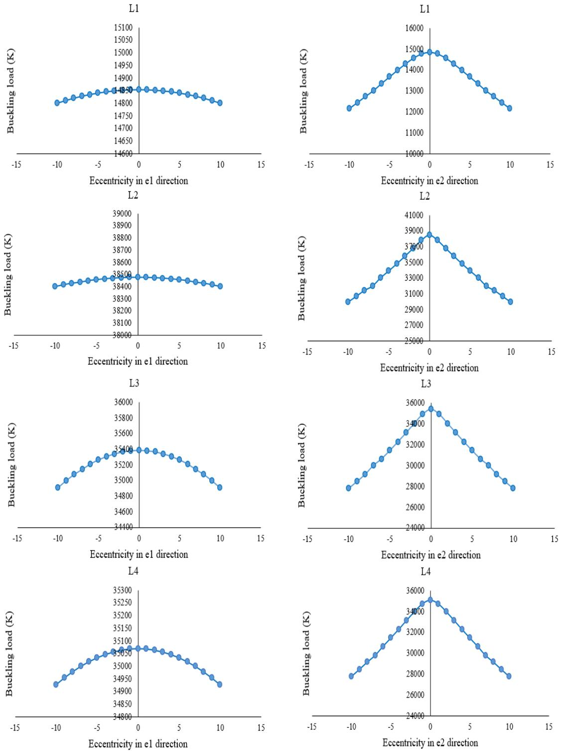
Fig. 8 Load eccentricity versus buckling load for box column
