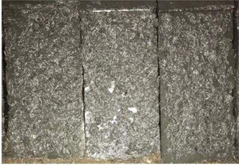
Fig. 16 Surface roughening of oblique shear specimen in rough interface group
