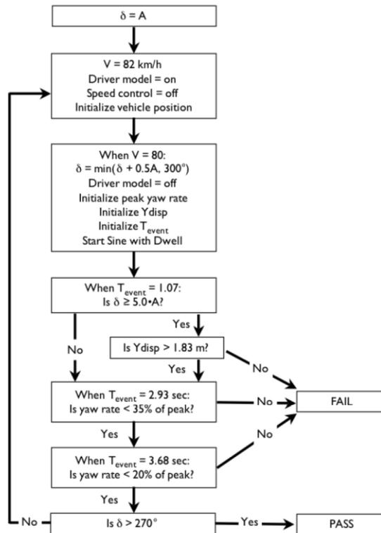
Fig. 10 The flow chart of FMVSS No. 126 test (CarSim 2011)
