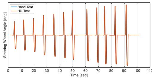
Fig. 11 The steering input for FMVSS No. 126 test
