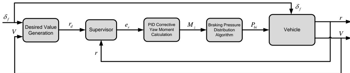
Fig. 17 The Basic ESC system block diagram
