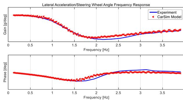
Fig. 4 Lateral acceleration/steering angle frequency response
