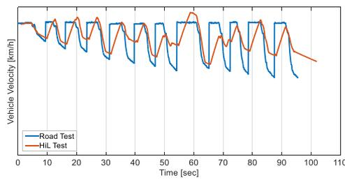
Fig. 12 Change of vehicle velocity over time for FMVSS No. 126
