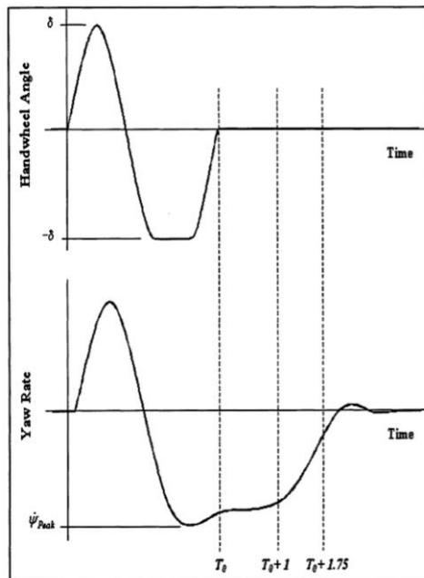
Fig. 9 Vehicle yaw rate change with respect to sine-with-dwell type steering angle input (NHTSA 2007)
