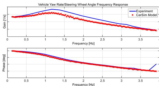
Fig. 5 Yaw rate/steering angle frequency response
