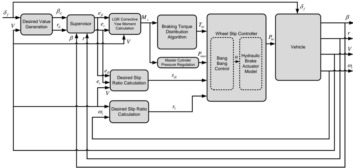
Fig. 18 The Integrated ESC system block diagram
