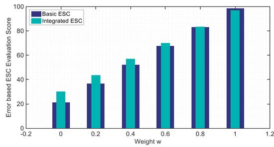
Fig. 19 Error based ESC evaluation scores for Fishhook test using different weights
