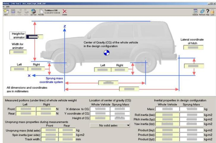
Fig. 1 The interface for vehicle dimensions in CarSim
